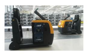
and diagnostics. The fuel cell can power a pallet jack for an entire 8-hour shift and can be refueled in 90 seconds, reducing vehicle and personnel downtime. Additionally, it operates in a range of temperatures, including freezer applications as low as -22°F. **Plug Power, 518-782-7700, plugpower.com.**
