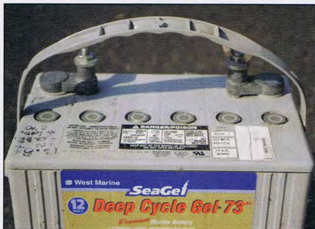
For a good, long life, big batteries need exercise and a smart charge cycle. (Photographs courtesy of WB6NOA).
