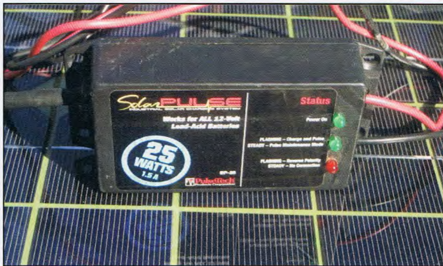
A Solar Pulse charging system sits on top of a solar panel during the tests in Arizona.
