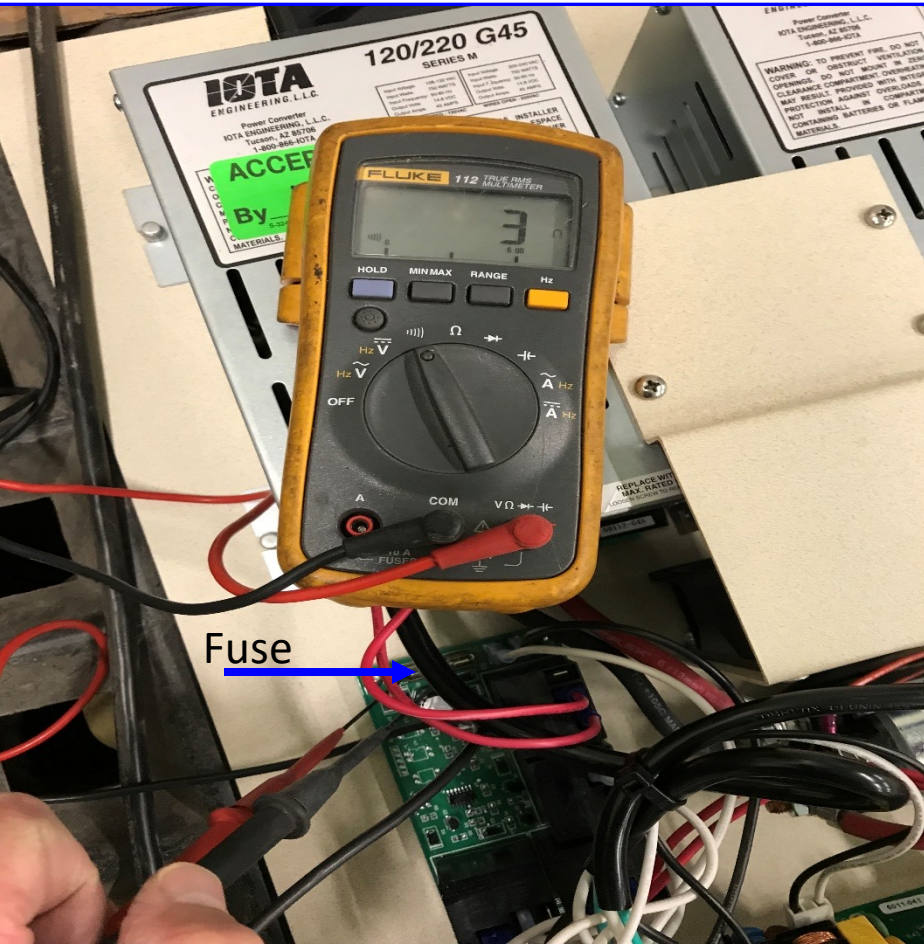
Test 2A: Sniffer Board Fuse Test.
