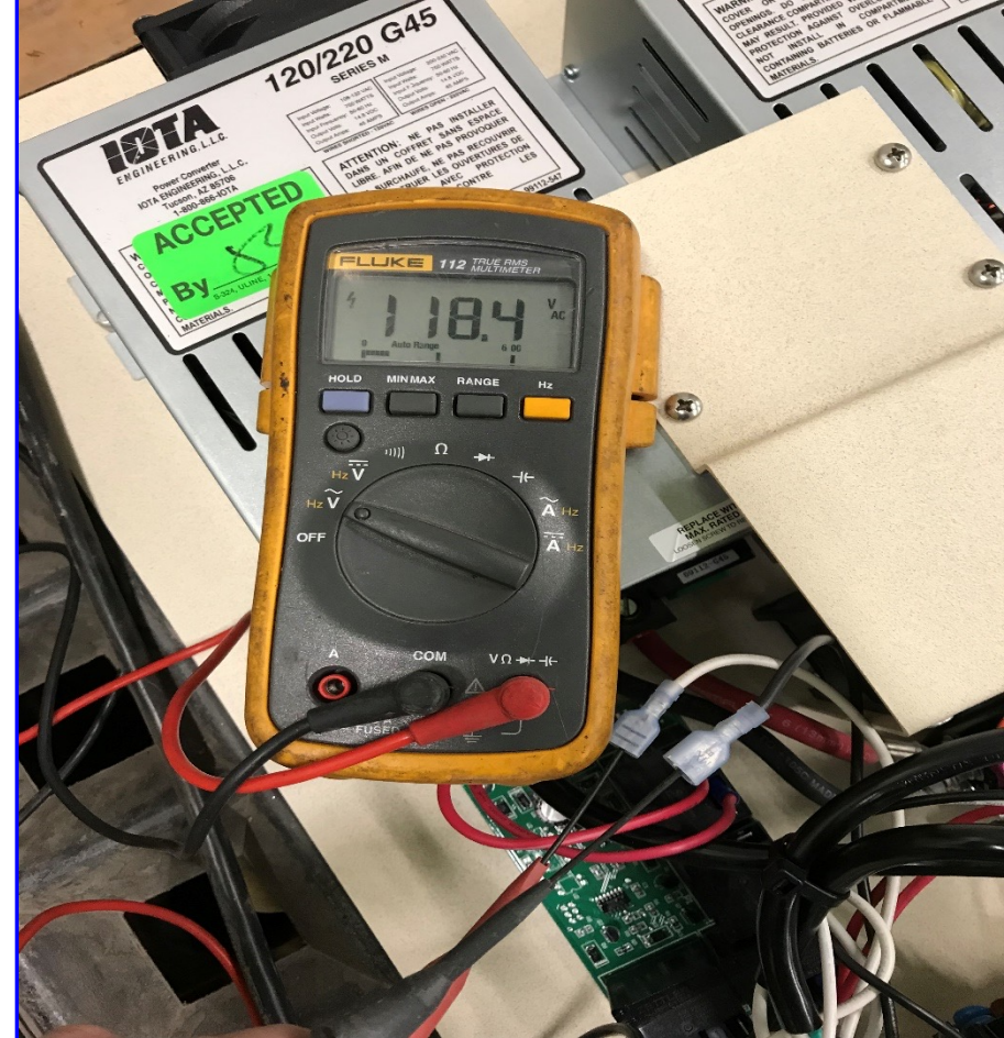
Test 2B: Sniffer Board AC input power test.
