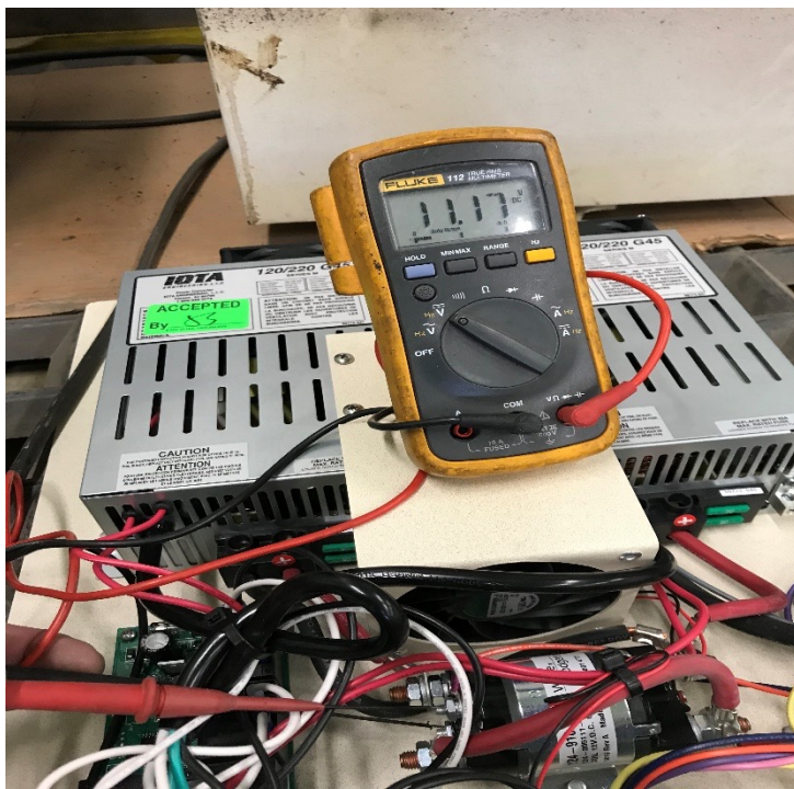
Testing activation VDC on 24V solenoid.
