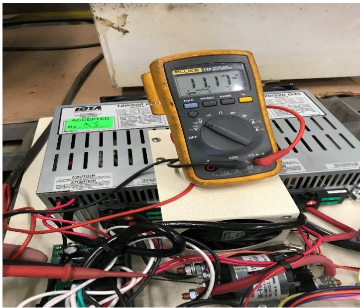
Testing activation VDC on 24V solenoid.
