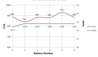
A full year after installation, the 6 batteries all showed a higher CCA (Cold Cranking Amp) and voltage reading than when they were brand new. In this case study, the Texas Fire Department extended the lifespan of their batteries and saw a 74% savings in battery costs over a 5 year period.
