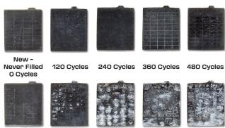
12-Volt Lead-Acid Batteries Charged with Typical Charger
