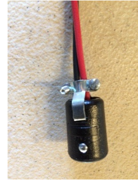
Drop Reel connection harness plug to Drop Reel quick disconnect plug.
