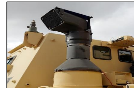
FMTV with 12 watt panel along with a Snorkel Mounting Kit.
