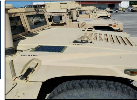
HMMWVs with 7.2 watt panels.
