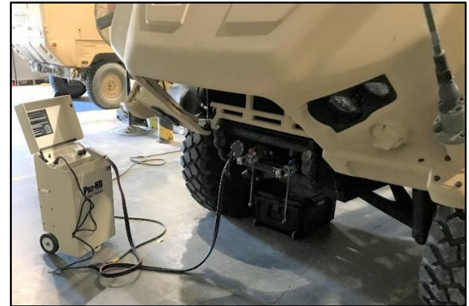
ProHD being used to charge the primary batteries on a JLTV.
