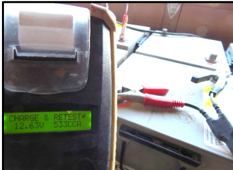
Example: Single Battery isolated, Tester Results: Charge and retest. 12.6VDC, 533CCAs
