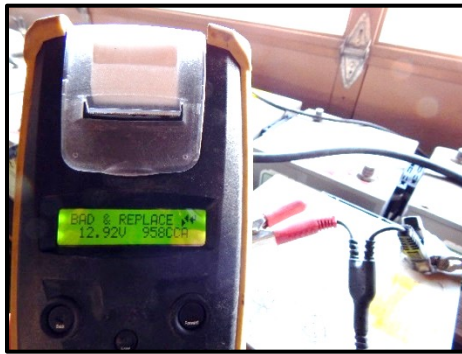
Example: Same Battery NOT isolated. Battery is paralleled with a bad battery and causes MUCH different reading. Tester Results: Bad & Replace. 12.9 VDC, 958 CCAs
