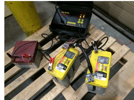
Example: Dual 24V Charger charging a 24V AGM battery and 2 - 12V batteries in series.
