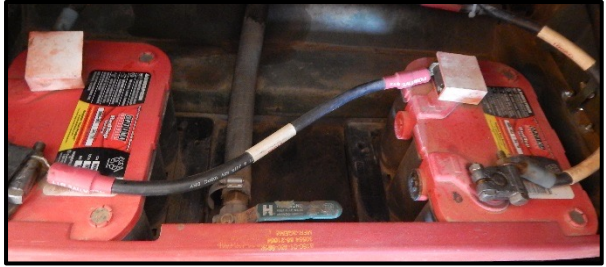
Example: Batteries are in series with another Battery. There will be no CCA nor Voltage from another battery.
