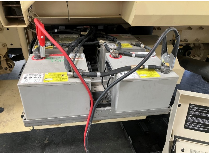
Example: Attempting charge the front 2 batteries on a 4 battery, series / parallel system.
