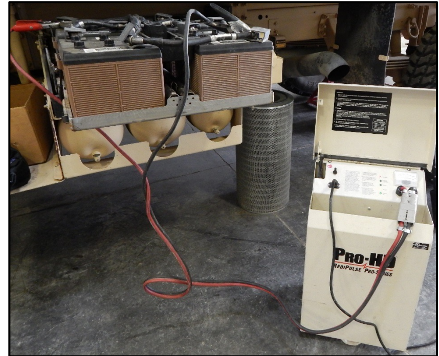
Example: Pro HD charging all batteries via clamps, and jump start or slave cables to other vehicle removed.
