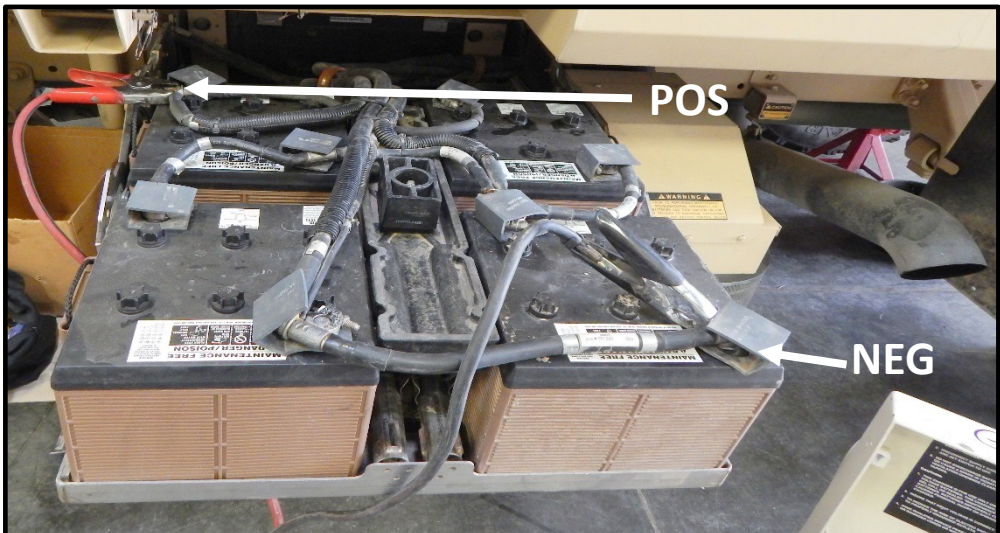
Example: Pro HD clamps hooked up to main POS and NEG clamps on an FMTV.
