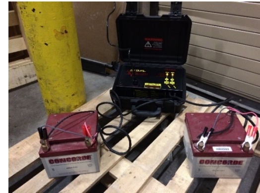
Example: Dual 24V Charger charging a couple 24V AGM batteries.
