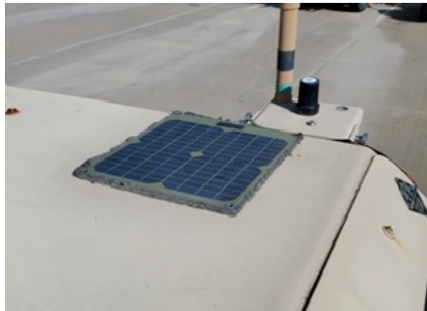
6.3 Watt Panel on M1152.
