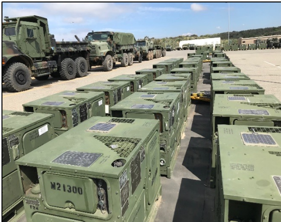
7-Watt Panels on Gen Sets.
