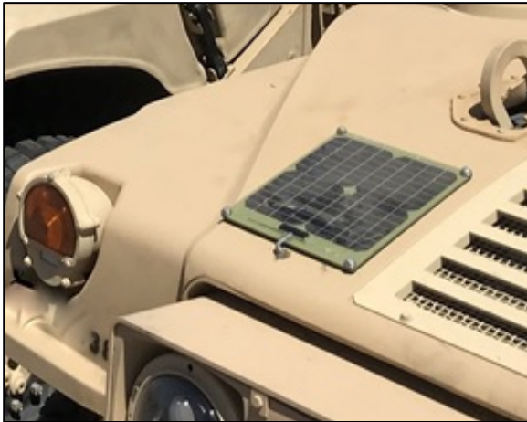
6.3-Watt hard mounted panel on HMMWV using 4 bolts, washers and locknuts.
