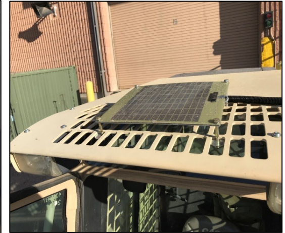
6.3-Watt Nato Plug SPCMS hard mounted on Case Skid Steer using 4 bolts, spacers, washers and locknuts.
