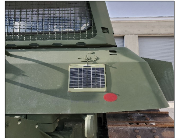
12-Watt Panel on Dozer.
