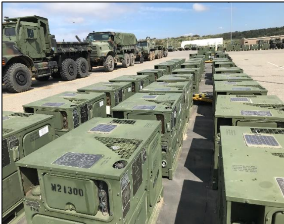
7-Watt Panels on Gen Sets.
