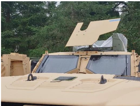
12-Watt Panel on a JLTV. This would be for the primary batteries.
