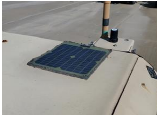
6.3 Watt Panel on M1152.
