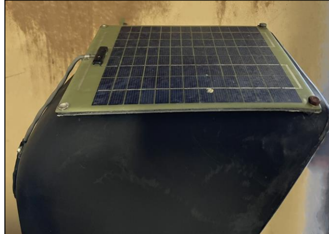
12-Watt 24V hard mounted panel on a M1083 MTV using RTV from the installation kit along with 2 bolts, washers and locknuts.
