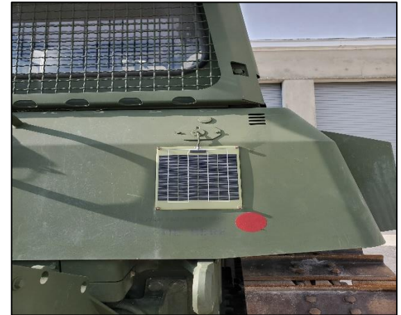
12-Watt Panel on Dozer.
