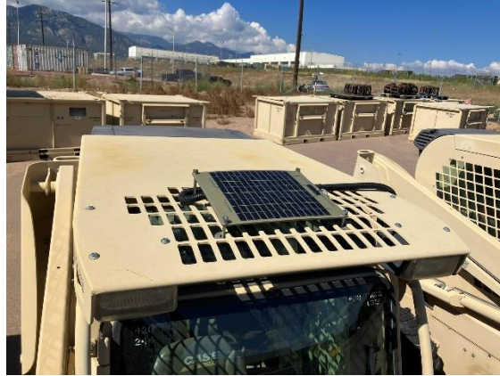
7-Watt Panel on a Skid steer.
