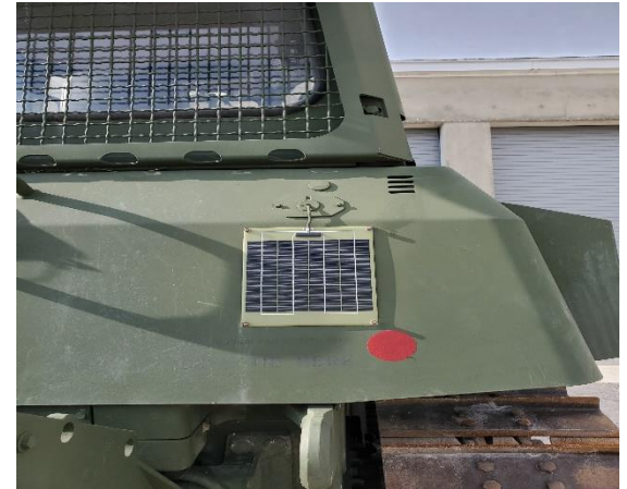
12-Watt Panel on Dozer.
