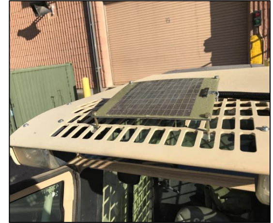
6.3-Watt Nato Plug SPCMS hard mounted on Case Skid Steer:
