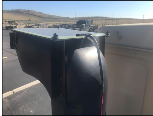
10-Watt Hard mounted with optional FMTV snorkel kit on M1083 MTV:
