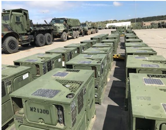
7-Watt Panels on Gen Sets.
