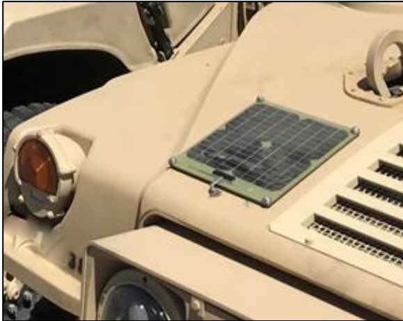
6.3-Watt hard mounted panel on HMMWV:
