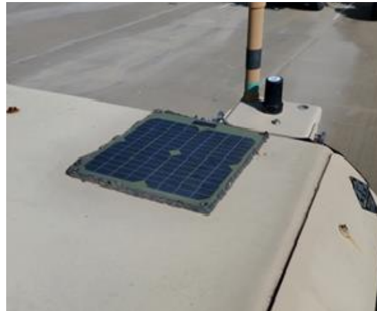
6.3 Watt Panel on M1152.
