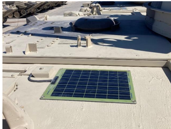
12-Watt Panel on NTC OPFOR Tracked vehicle.
