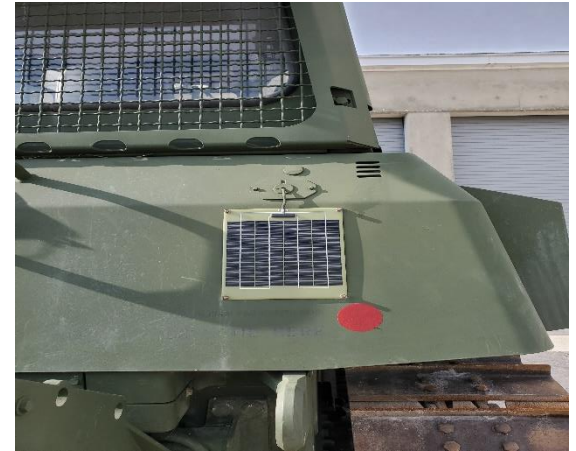
12-Watt Panel on Dozer.
