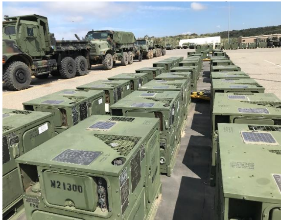
7-Watt Panels on Gen Sets.
