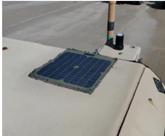
6.3 Watt Panel on M1152.
