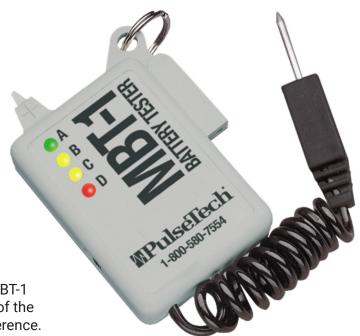
When individual batteries are wired in series, the MBT-1 will give the operator an accurate reading of each battery without the need to disconnect the batteries, translating to saved time and money. When individual batteries are wired in parallel, the MBT-1 will test both batteries together and give you an indication of whether the pair is weak relative to others tested. Parallel batteries should be disconnected to test individually. Reverse polarity and over voltage protected.
