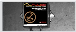
The circuit box can be mounted using any of the following methods: Two round-head screws, industrial adhesive, heavy-duty dual lock or double-sided tape (not included). After cleaning the install area, mount the box close to the battery so that the lugs can reach the terminals. DO NOT attach it to the battery itself. Also make sure the box is located in a location where it won't be disturbed and the LED is visible.
