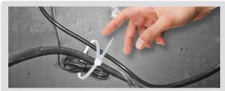
If needed, use plastic cable ties (not included) to secure the circuit box wires to the battery cable or other secure area near the battery. This will keep the wires from being damaged or interfering with any moving engine parts.
