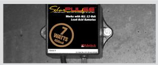
The circuit box can be mounted using any of the following methods: Two round-head screws, industrial adhesive, heavy-duty dual lock or double-sided tape (not included). After cleaning the install area, mount the box close to the battery so that the lugs can reach the terminals. DO NOT attach it to the battery itself. Also make sure the box is located in a location where it won't be disturbed and the LED is visible.
