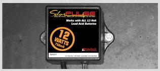
The circuit box can be mounted using any of the following methods: Two round-head screws, industrial adhesive, heavy-duty dual lock or double-sided tape (not included). After cleaning the install area, mount the box close to the battery so that the lugs can reach the terminals. DO NOT attach it to the battery itself. Also make sure the box is located in a location where it won't be disturbed and the LED is visible.
