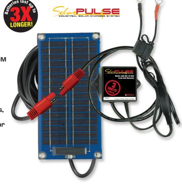
The 3-watt SolarPulse charges, maintains and desulfates 12-volt batteries in vehicles and equipment that are stored and used outside, replacing the power loss from electrical accessories that occurs even when the ignition is switched off. Rated at 240 mA, the SP-3 is reverse polarity protected. At just 4.70" x 9.45" x 0.25", it can be flush mounted with the smallest possible footprint.
