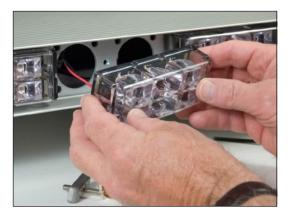
**6.** Reverse Step 1 above to reinstall lamp. Torque to 14 inch-lb.
