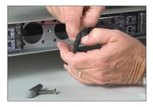
**3.** Using a fingernail pull up on the connector lock clip and disconnect the lamp.
