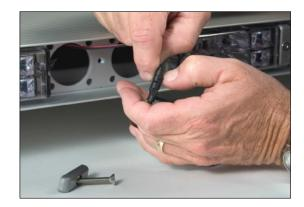
**3.** Using a fingernail pull up on the connector lock clip and disconnect the lamp.
