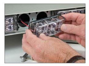
**5.** Put the lamp into position making sure the wires go inside the lightbar through the hole.
