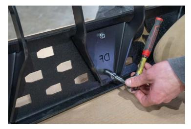
ATTACH BRACKETS TO STEPS USING (2) 1/4"-20 STAINLESS FLAT HEAD BOLTS (J) AND (2) 1/4"-20 ZINC NYLOCK NUTS (K) WITH QTY(2) 1/4" WASHERS (L) UNDER EACH NUT, PER BRACKET.
