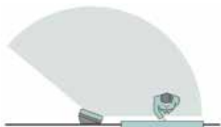
Installation with Bracket: 15° Angle
