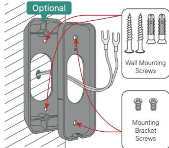
Feed the power cable from the inside through the drilled hole in the center and through the mounting plate and bracket (optional). Now fix the mounting plate and bracket (optional) to the wall.
