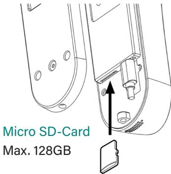
If you want to install a SD-Card for automatic video recording, it is recommended to insert it into the device before mounting. The SD-Card slot is located at the bottom of the back of the device.
