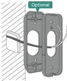
Place the mounting plate and mounting bracket (optional) at the mounting location and feed the existing doorbell wires through the hole in the center of the mounting plate.
