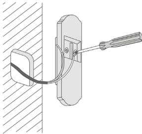
Turn off the main power switch (fuse) before connecting!
