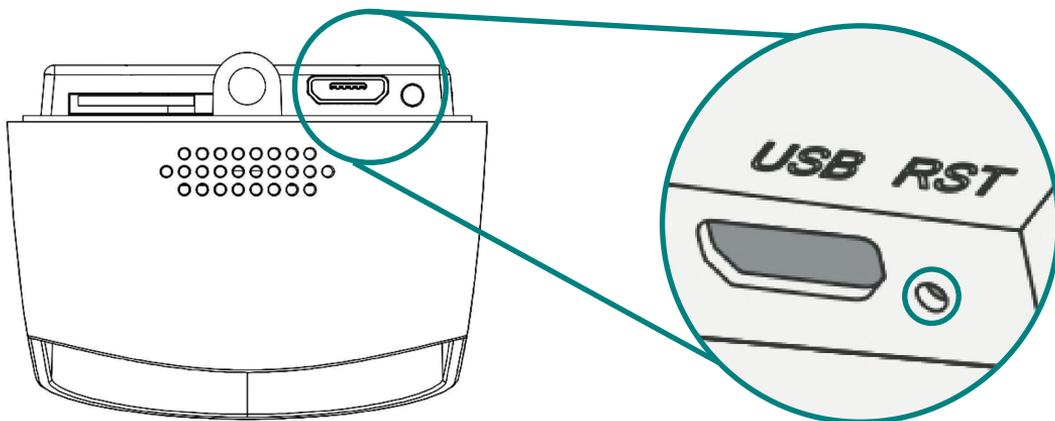
Take the enclosed reset pin and carefully press in the reset button (see illustration above) for about 5-8 seconds. After the video doorbell has been successfully reset to the factory settings, a signal tone will sound. The indicator LED will flash red after the reset.
