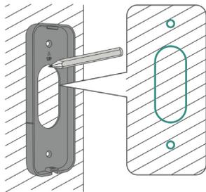
Hold the mounting plate at the mounting location and mark the drill holes with a pencil.
