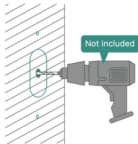
Drill the holes for the mounting plate at the marked locations. Drill another hole in the center of the mounting plate to feed the power cable through from the inside.
