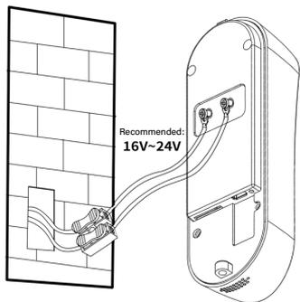
Connect the existing doorbell wires (AC12-24V) to the contact points of the Cardea and fix them with the enclosed screws.
