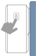
**Connection Mode:** Press the volume button for approx. 4 seconds until the LED indicator lights up.
