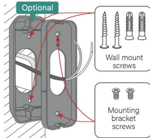
Mark the drill holes and drill the holes at the marked positions. Now fasten the mounting plate and the mounting bracket (optional) with the enclosed screws.
