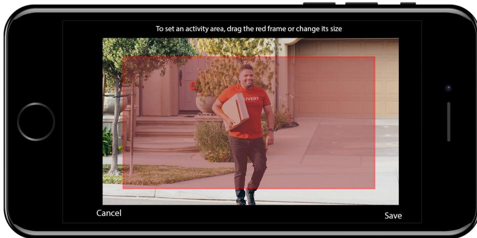
Select the desired detection area with your finger. Movements are only detected in the area marked in red. After you have marked the desired area, press 'Save' in the lower right corner.
