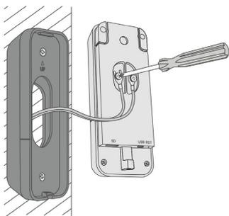
Connect the power cable to the video doorbell using the screws provided.
