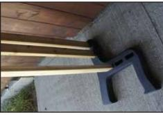
2. Lay one of the bench ends on the ground and insert each of the pieces of lumber into the slots. Make sure the wood is flush with the outer side of the bench end.
