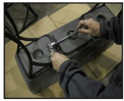
6. Repeat step 5 on 2nd bolt, assembly should now be rigid and secure.
