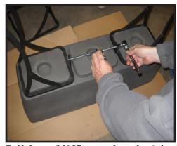
5. Using a 9/16" wrench and ratchet, tighten the first bolt as show, ensure not to over tighten the bolts.
