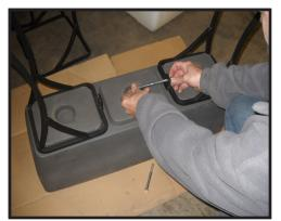
2. Place a washer on each bolt and slide bolt into opening of leg as shown above.
