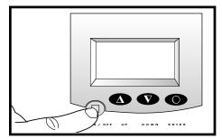
**NOTE:** To turn the machine OFF, press the ON/OFF button. The machine beeps twice and turns OFF.
