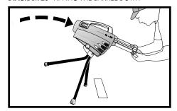
**NOTE:** If the cup is out of reach, position the machine so that the barrel faces down. Gravity helps the cup settle forward.
