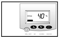
IMPORTANT: Changes to the power level settings can only occur when the compressor is not running. Pressing any button when the compressor is running, activates an emergency shut down.
