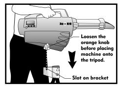
2. With the barrel of the machine fairly level, place the front edge of the cutout against the front of the tripod's mounting bracket. Lower the machine into place. See Diagram 8.
