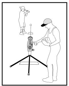
To adjust the pitch height in the strike zone, slightly increase or decrease the power level. If the power level is changed significantly, you will need to adjust the pitch angle (elevation). Refer to "Determining the Pitch Angle" on page 10.
