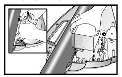
Remove the battery connectors by lifting the battery slightly from the case bracket to gain access. Gently, slide both connectors off the terminals of the old battery. Pull on the connectors, not on the wires.
