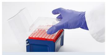
The refill process takes only seconds. Tips can now directly be used or autoclaved before usage\*.
