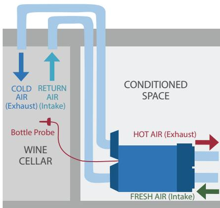
\* Venting to the exterior may require the addition of compressor heater (temps below 40°F) and fan cycling switch (temps below 20°F).
