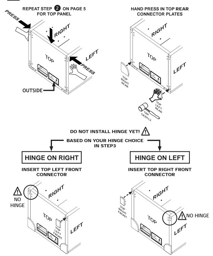
TAP IN CONNECTORS TIGHTLY (NO GAP) WITH CLOSED HAND OR RUBBER MALLET (SAVE REMAINING CONNECTOR PLATES IF YOU DECIDE TO CHANGE HINGE SIDE)
