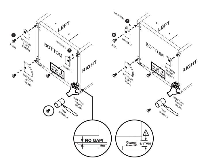
TAP IN CONNECTORS TIGHTLY (NO GAP) WITH CLOSED HAND OR RUBBER MALLET SCREW IN ALL LEGS LEAVE MIN 1/4" SPACING ON ALL LEGS
