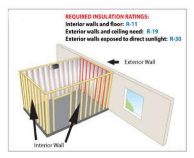
It is important that all walls, joints, doors and windows, electrical outlets and/or switches, pipes, vents and light fixtures be sealed to prevent air and moisture from entering the cellar. If there is a leak in the cellar, the cooling unit will build up excess condensation.
