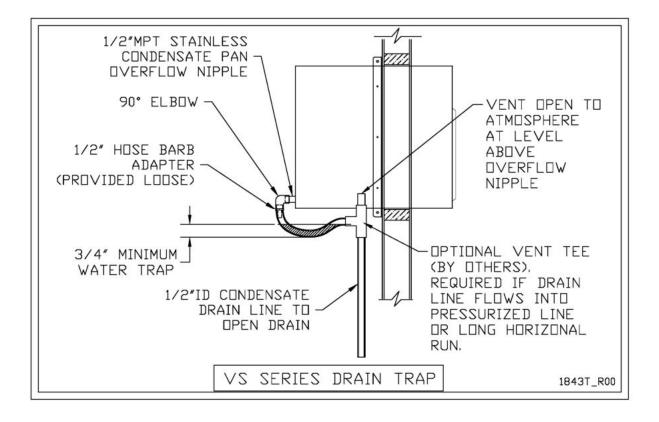
As shown above, the drain line should drop, then rise (but stay below the height of the fitting), and then drop again into a drain or bucket. Then, fill the trap with water. The condensate trap will allow any excess moisture inside the cooling unit to overcome the static pressure and flow out of the drain line.
