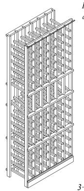
$1\frac{1}{2}$ " Crown moulding attached to top of rack  $3\frac{1}{4}$ " baseboard attached
