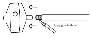
Make sure to attach the stem to the main body by first threading the cable through the stem and then Screwing together to securely attach using glue provided. Apply the glue to the thread shown in diagram above.
