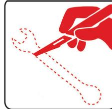
Lightly press on the item, so it doesn't move. Trace cut around the item, keeping the knife perpendicular and as close to it as possible.
