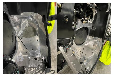
**Step 9:** Install the new silencers onto the sled, we suggest using a small film of high temp silicone around the exhaust donut gasket.
