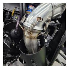
**Step 12:** Install the EGT sensor into the new silencer. Tighten with a 17mm wrench.
