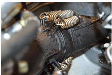
Install the turbo coolant lines. The 90 degree line goes to the coolant bottle, and the straight line goes directly to the cylinder head. You will not run coolant through the throttle bodies with the turbo kit. The lines come installed on the turbocharger and must be re installed the same way. 90 line towards the side panel and straight line towards the engine.
