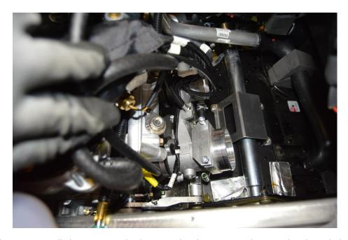
Intercooler Kits. Install the two supplied Two Hole Aluminum Tabs into the throttle body Boot. Remove the factory 8mm bolts, and install the tab using the supplied socket head bolt. You will install one tab on each side of the boot. Located the Intercooler airbox and install it onto the throttle bodies. Fasten to the engine using the Supplied Bolts, Nuts, and O rings. Use picture for installation. Tighten the nut so it start to smash the o ring. Do not over tighten.
