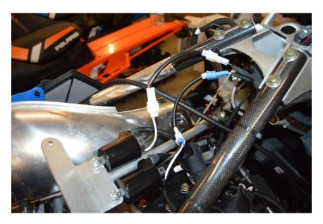
Remove the two oil lines from the pump, You will remove the two lines in pictures. Caution you must install these lines correct to ensure proper engine lubrication.
