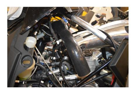
Install the hood plenum. And install the coil bracket behind the ecu.
