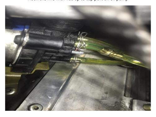
Locate the Turbo Oil Line. Using a syringe fill the line with Polaris VES oil. Connect one end of the Turbo Oil line to port direcly below the line with TEE of the electronic oil pump. Use the stock oil line clamp on the pump side.
