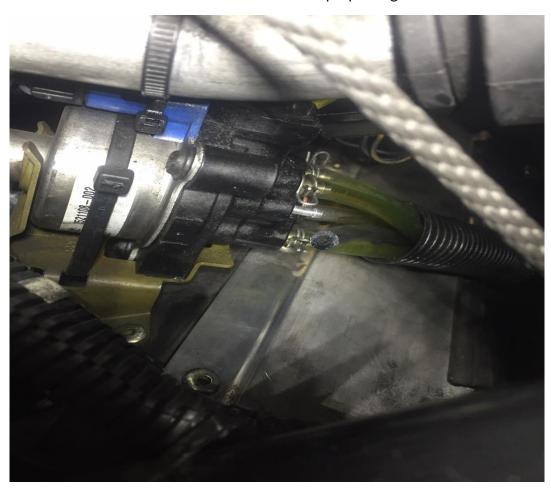
Push the first line you remove into tee. You will not have to use any clamps on the lines that connect to the TEE ( it's a push lock connection and no clamps are required.
