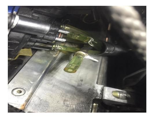
Locate a syringe, then fill it with Polaris 2 stroke oil and fill the 2 lines with oil so the air bubbles are gone.
