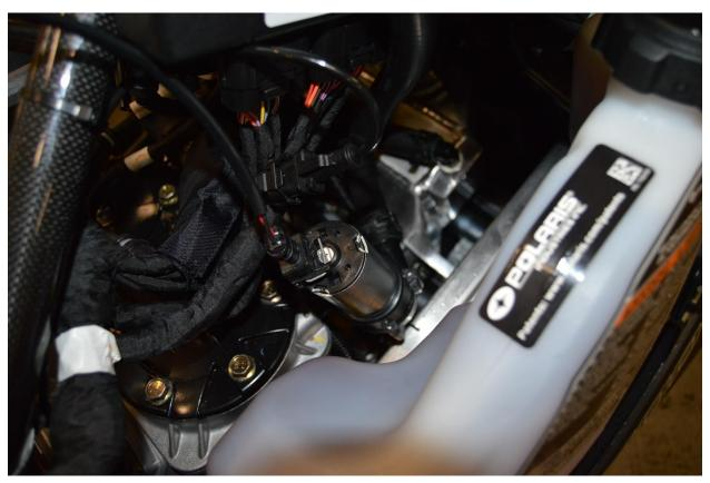
Install the Turbocharger assembly onto the snowmobile. Install the stock rubber grommets onto the turbo assembly and lower bulk hed. Use the 4 long springs to connect the turbo to pipe. Using the Long Muffler hanger spring, connect the turbo to the hanger bar to the tab welded on the down pipe.
