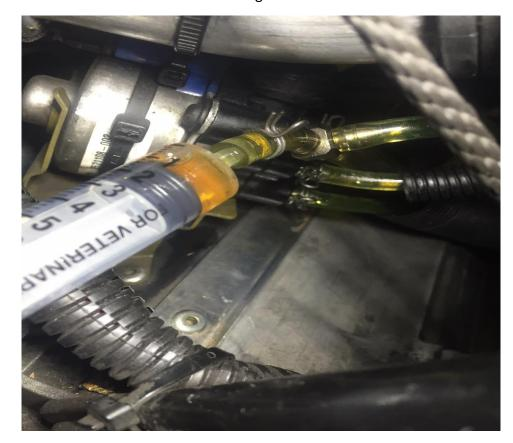
Hook the line with TEE up to top port on oil pump
