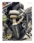
**Step 8:** Set the factory wastegate elbow in place and align the wastegate connections. Once aligned tighen the v-band clamp at the base and then the one going to the factory elbow. Install the main v-band clamp to the turbo.
