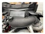
**Step 2:** Remove the turbo air intake adapter ( 2- plastic push darts and hose clamp) Carefully lay it to the side and leave the sensor attached.
