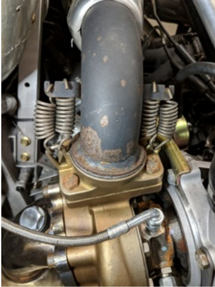
Double Spring the Turbo to Pipe tabs using the supplied 2" Exhaust Springs.
