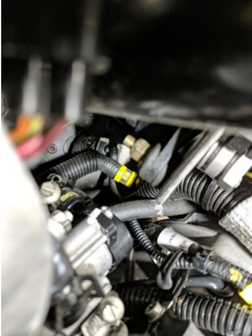
Coolant Line coupled to the OEM coolant line.
