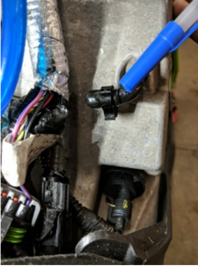
Cap The Oil Tank Port using the Supplied Vacuum Cap and Clamp
