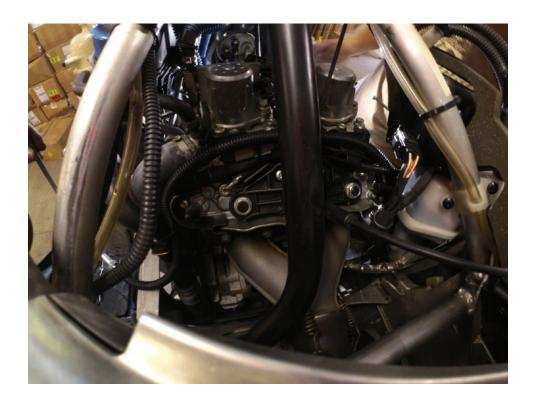
Using a syringe prime the turbo oil line. Once primed install the line onto the lower port of the pump and fasten with the supplied spring clamp. Make sure all the lines are filled before connecting them to the pump.
