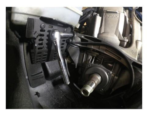
Remove the oil pump guard. Than remove the two oil lines that feed the rave valves from the oil pump. They are fastened to the pump with the pinch clamps. A side cutter works good to cut them.
