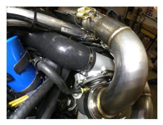
Double spring the turbocharger to pipe using the supplied springs. Also make sure every spring is doubled up on each tab. There are three tabs on the Y Pipe, each tab needs two springs.
