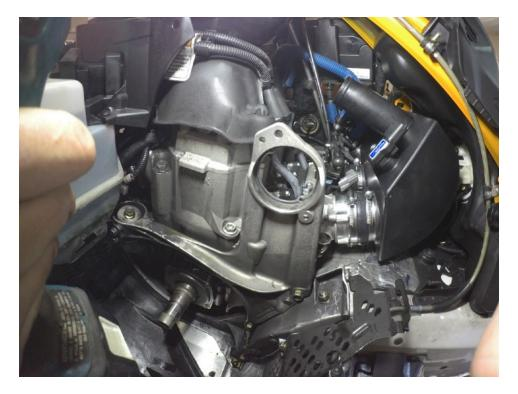
Route the Cold Air Intake Tube through the chassis. Also notice the Reflective heat tape we install onto the frame bar. This will prevent the vent hoses from being melted. We highly suggest installing multiple layers of heat tape to prevent any damage.
