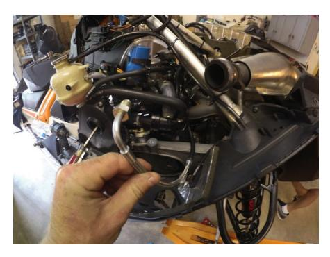
Notice the line routed above the rave valves. Properly fasten these so they don't interfere with the operation of the rave valves.
