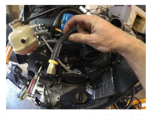
Install the long coolant hose onto the coolant tank, fasten with the supplied clamp.
