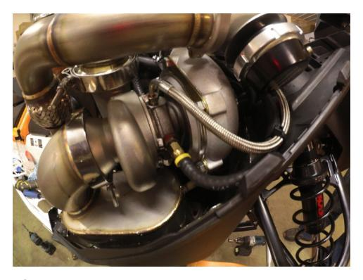
Install the EGT probe into the new muffler.
