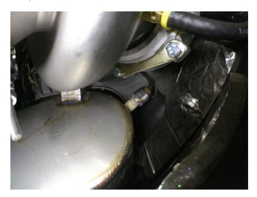
Install the silicone charge tube onto the turbocharger and fasten with the supplied clamp.
