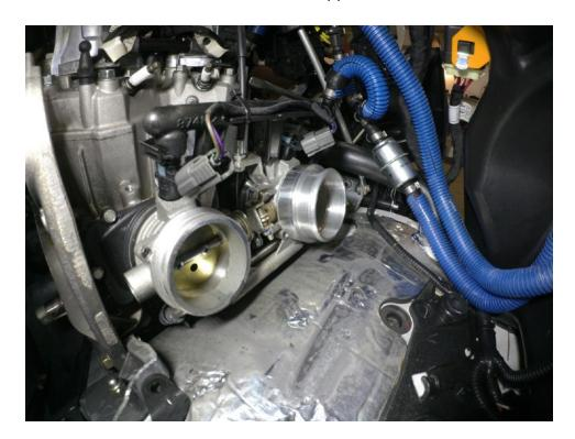
Install the Airbox on to the throttle body adapters. Be sure to secure all the hose clamps.
