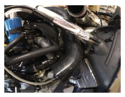
Install the Turbo Coolant lines. Remove the hose from the top of the coolant tank and install the supplied push lock fitting into the end of the hose. The coolant lines come installed onto your turbocharger assembly.
