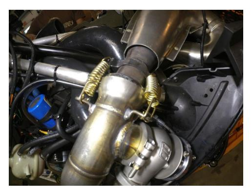
Install the charge tube onto the air box and fasten with the supplied clamp. Also locate the Map Sensor extension harness and clip it onto the map sensor located in the airbox.
