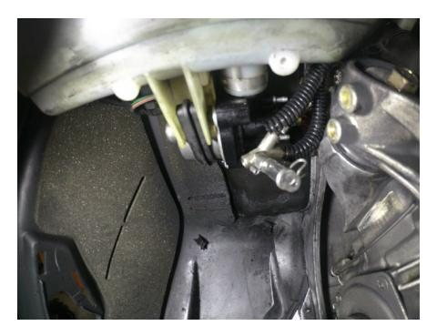
Once the oil lines are installed onto the TEE, use a syringe to inject two stroke oil and prime the lines. Use enough oil to get all the air bubbles out of the lines. Once the lines are full install the single end of the TEE onto the top port of the oil pump. Fasten with the supplied spring clamp.
