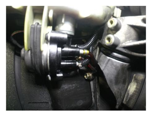
Install the supplied oil line TEE, put one oil line on each barb of the tee, and fasten with the supplied pinch clamps.
