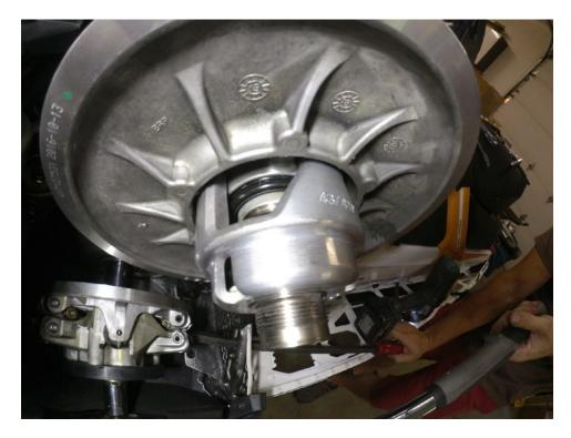
Install the belt and check for proper belt deflection. Make sure to check your belt deflection after a few minutes of operation.
