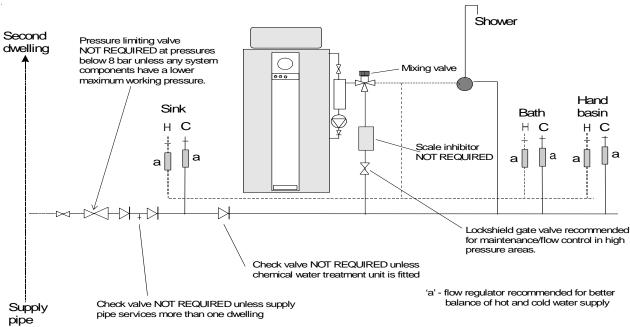
Figure 1.1 Typical hot and cold water distribution network
