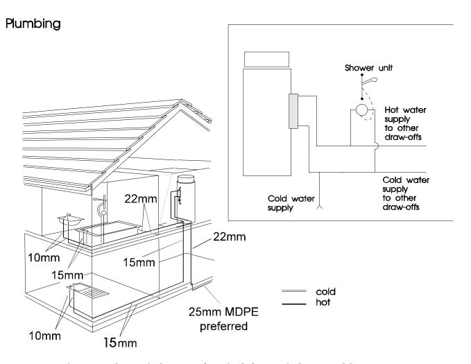
Fig 2.1 Schematic layout of typical domestic hot & cold water systems.
