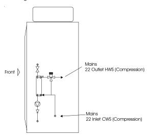
Fig 3.1 PulsaCoil III pipe connection arrangement
