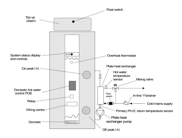
Figure 1.2 Standard PulsaCoil III Package
