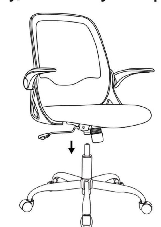
\* Caution: If the Air Rod (6) doesn't insert to Base Plate (8) firmly, it's likely to fall of when the chair raises up.
