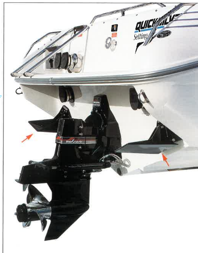
Figure 8-35 Kiekhoefer K-Planes™ provide efficiency, comfort, and control.
