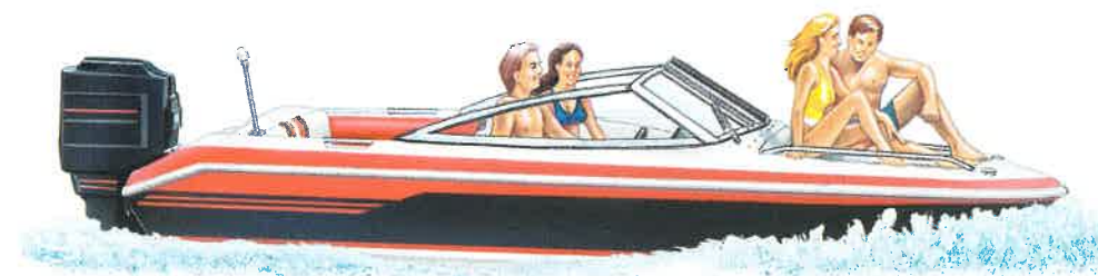
Figure 8-37 Weight concentration far forward impairs performance, handling, and operator visibility.
