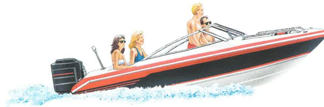
Figure 8-36 Weight concentration far aft is often preferable for top speed but still has some disadvantages.
