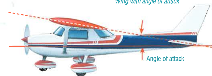
Figure 4-25 Angle of attack creates a pressure difference resulting in lift.
