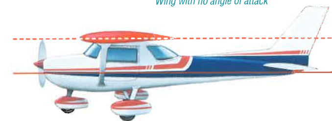
Figure 4-23 No angle of attack results in no lift (will not fly).
