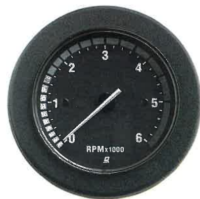
Figure 8-31 A tachometer measures engine revolutions per minute (RPM).
