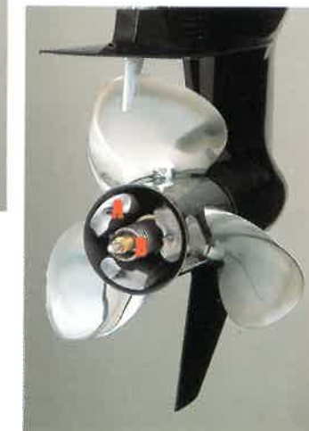
Figure 6-15B (below) A: Weight arms B: Prop nut and torsional spring
