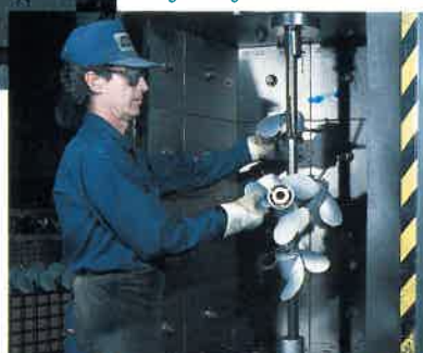
Figure 5-6 Shot blasting, before and after grinding for surface finish
