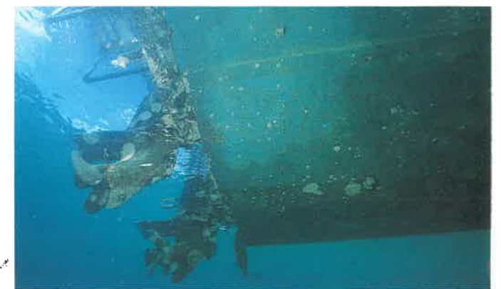
Figure 8-43 Marine fouling on the boat bottom and drive units.
