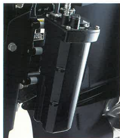
Figure 8-30A (right) RideGuide outboard power steering pump motor/accumulator
