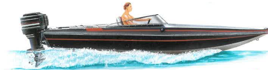
Figure 8-19 Engine or drive trimmed "in" (bow too low).
