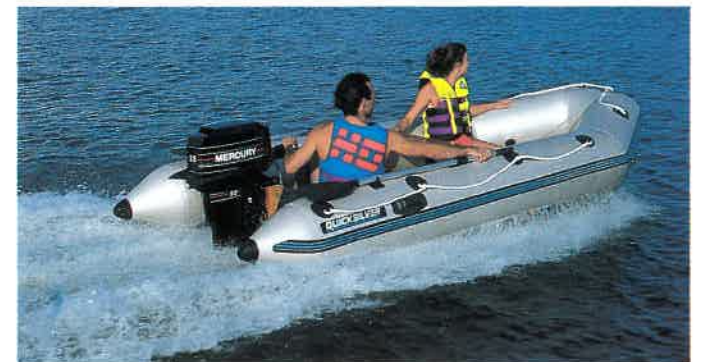
Figure 7-24 Inflatable boat with inflatable keel, rigid floor boards and flexible material bottom.
