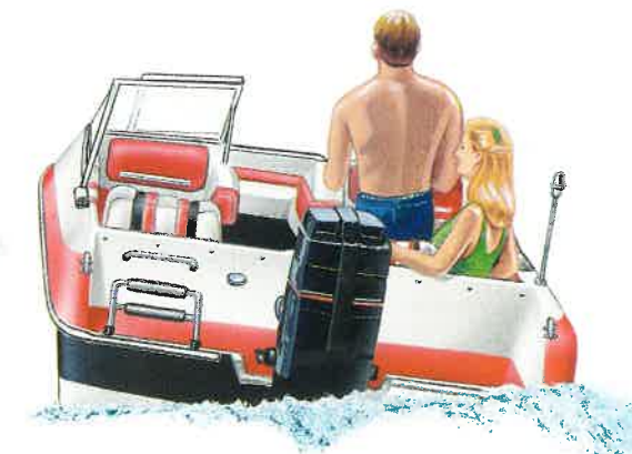
Figure 8-38 Uneven lateral weight distribution can produce severe listing.
