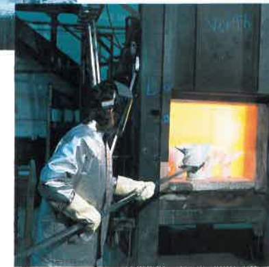
Figure 5-13 Preheating stainless steel propeller molds
