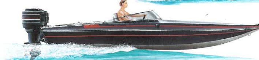
Figure 8-21 Engine or drive properly trimmed.
