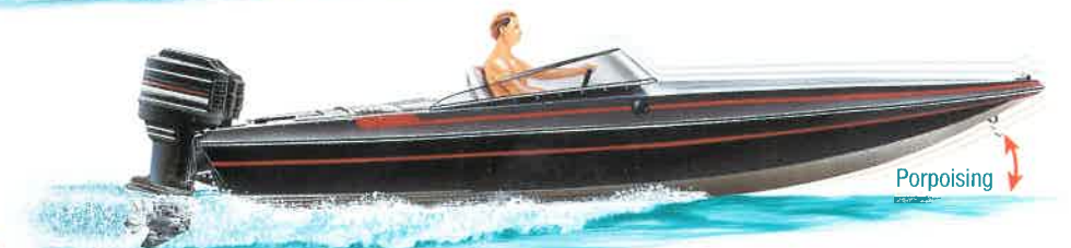
Figure 8-20 Engine or drive trimmed "out" (bow too high).
