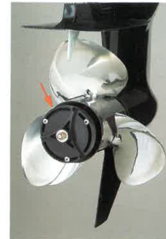
Figure 6-15A (left) Rotary cam controls the shift tension and thereby the shift point.
