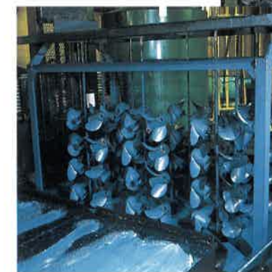
Figure 5-10 Electro-deposition painting of aluminum propeller
