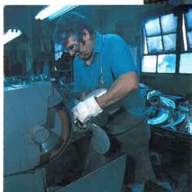
Figure 5-7 Grinding of aluminum propeller
