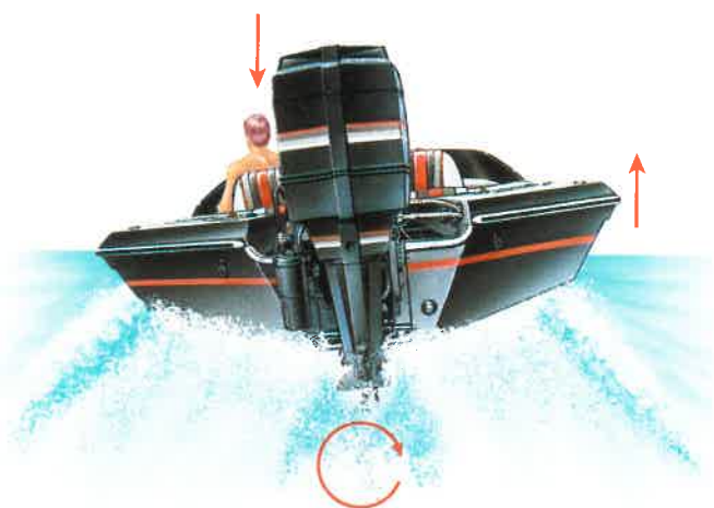
Figure 8-5 Driver on port side enhances boat roll (right-hand rotation propeller).
