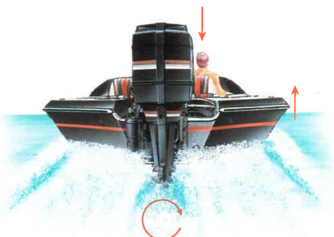
Figure 8-6 Driver on starboard side balances boat roll (right-hand rotation propeller).
