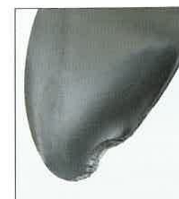
Figure 8-42 A damaged propeller blade significantly reduces performance.
