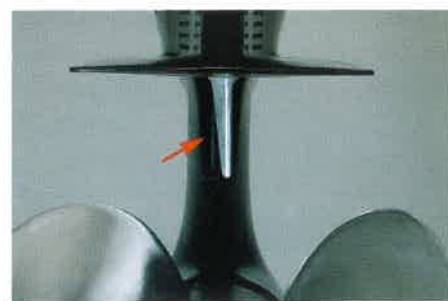
Figure 8-27 Adjustable trim tab can be set to help counteract steering imbalance when antivibration plate is at or very little above boat bottom. Illustration shows trim tab trailing edge set to the right to help offset pull to the right as in Figure 8-23.
