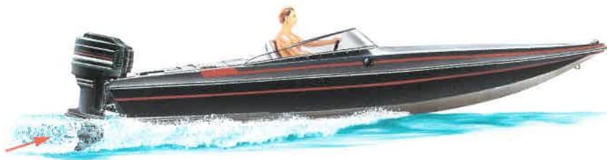
Figure 4-17 Ventilation: air being sucked into propeller
