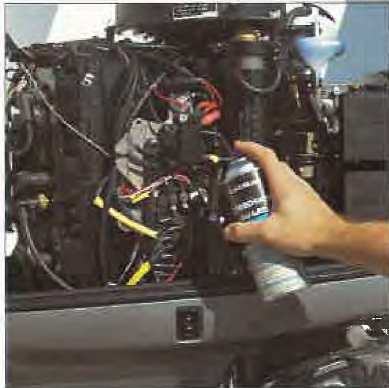
Figure 4-2 Spray powerhead and all electrical connections with Quicksilver Corrosion Guard
