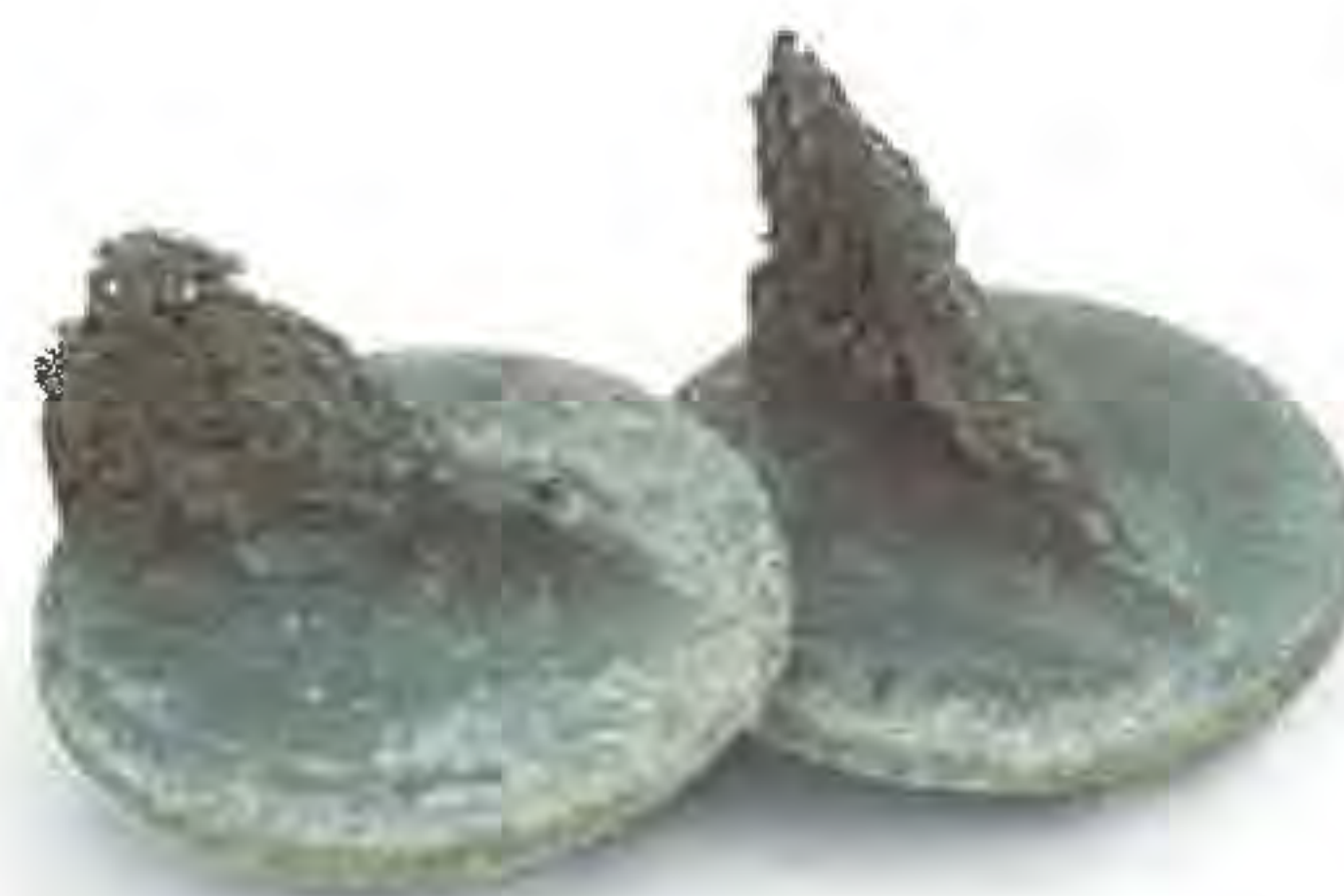
Figure 4-3 Inspect sacrificial anodes regularly and replace when 50% consumed
