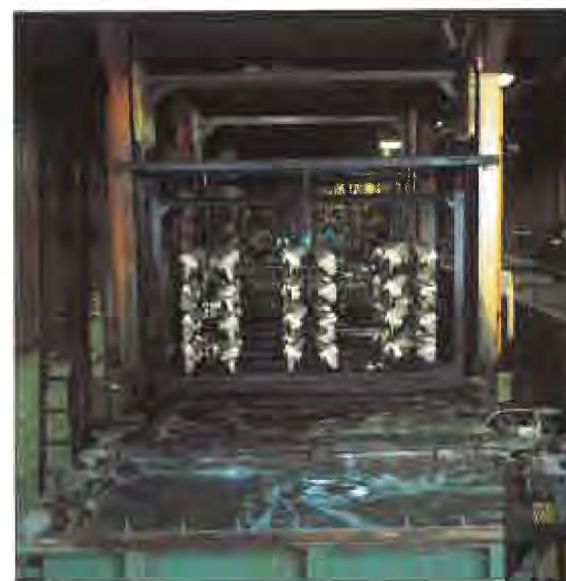
Figure 2-1 Aluminum alloy parts being chemically cleaned
