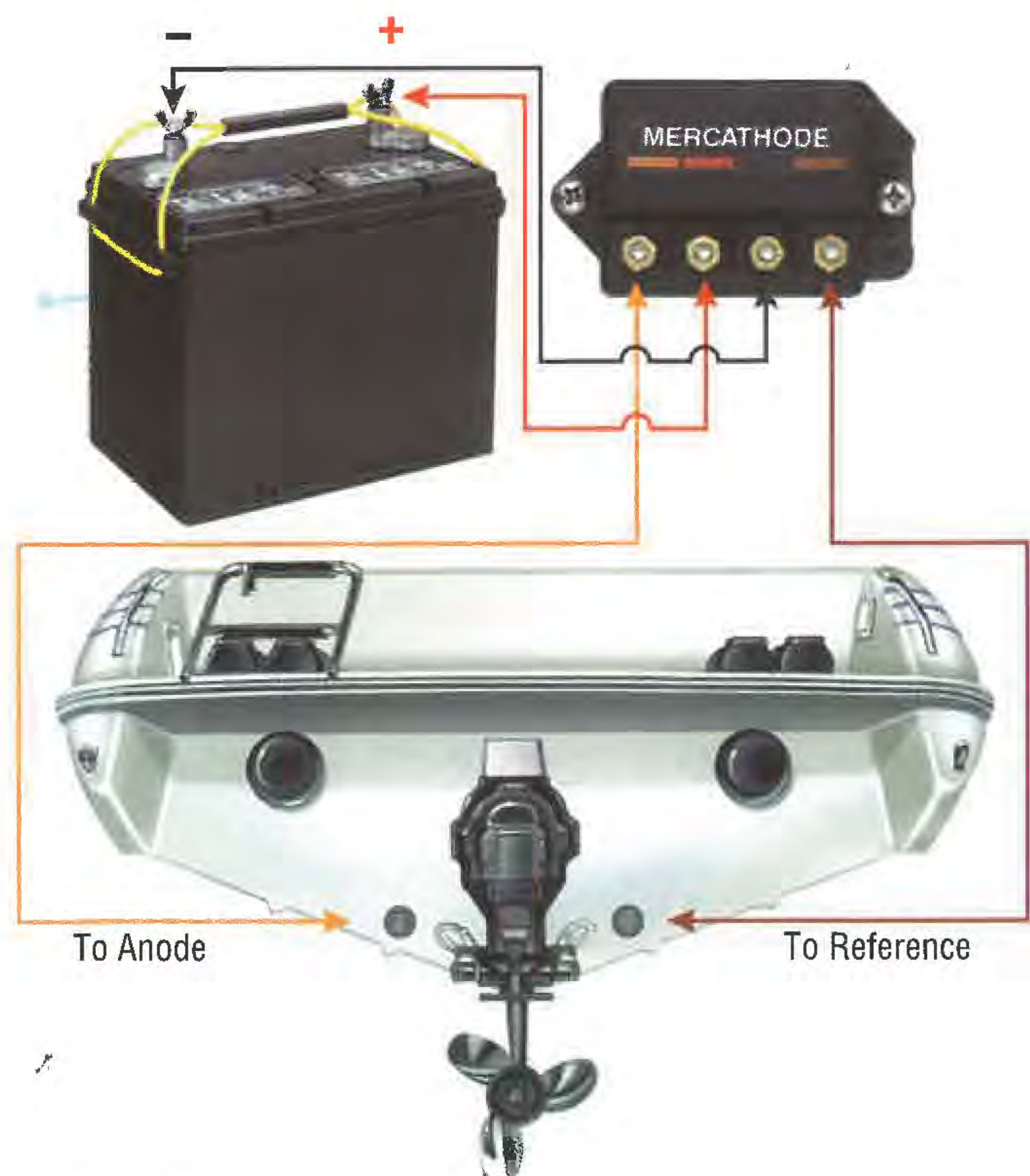
Figure 2-13 Quicksilver MerCathode System installation
