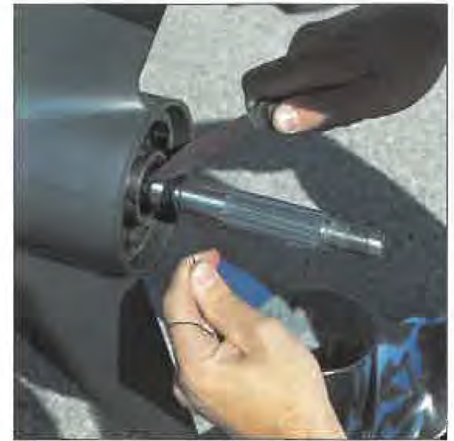
Figure 4-5 Check prop for fish line
