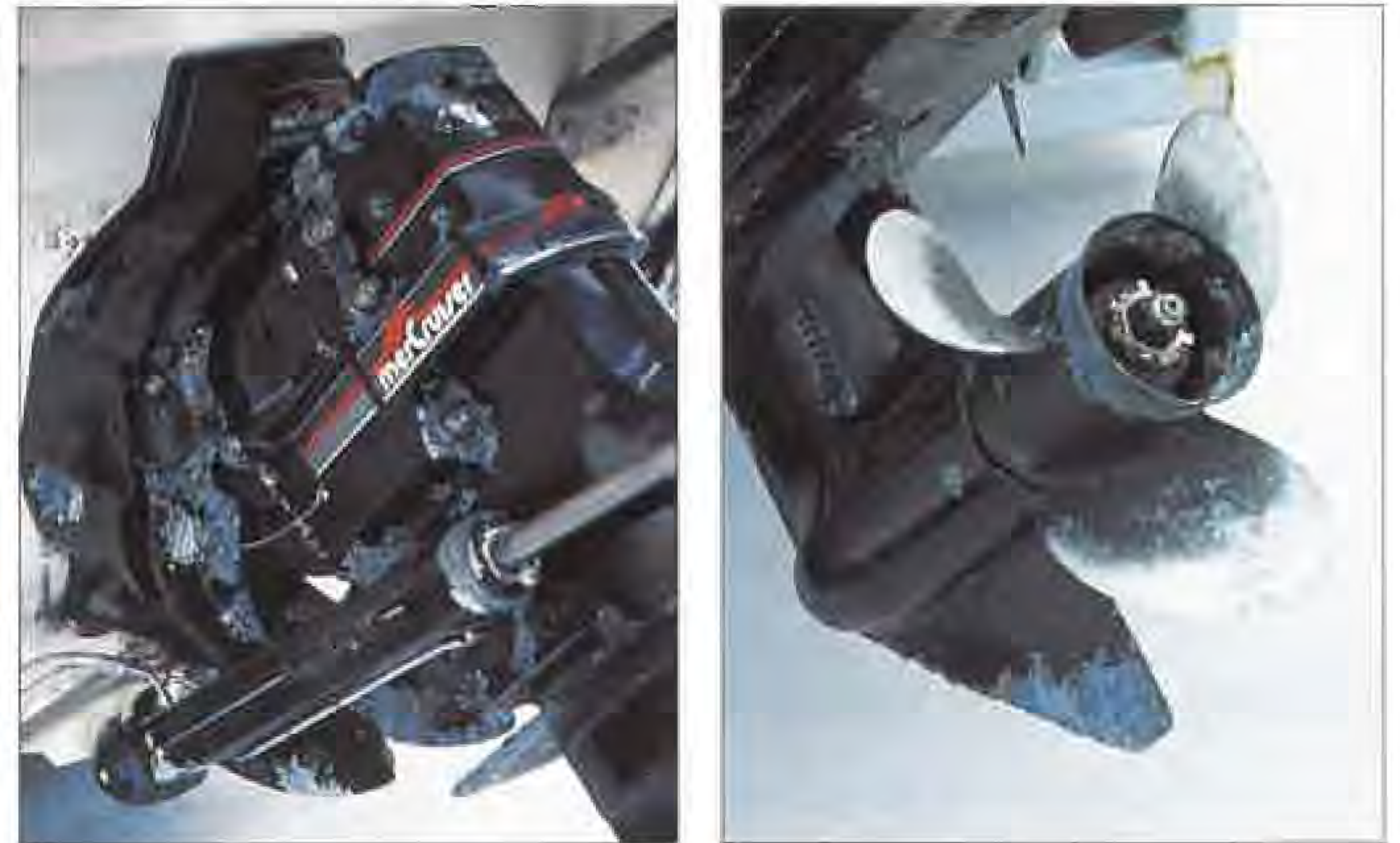
Figure 1-3 Corrosion on aluminum lower unit and propeller
