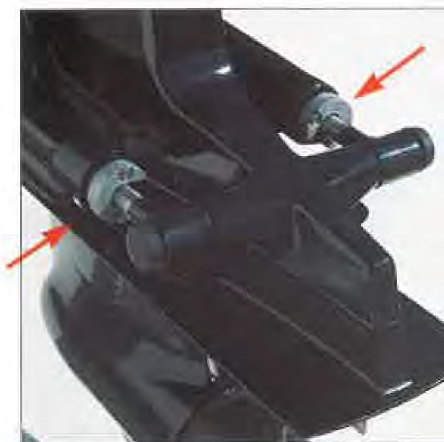
Figure 2-6 Sacrificial trim cylinder anode on trim cylinder
