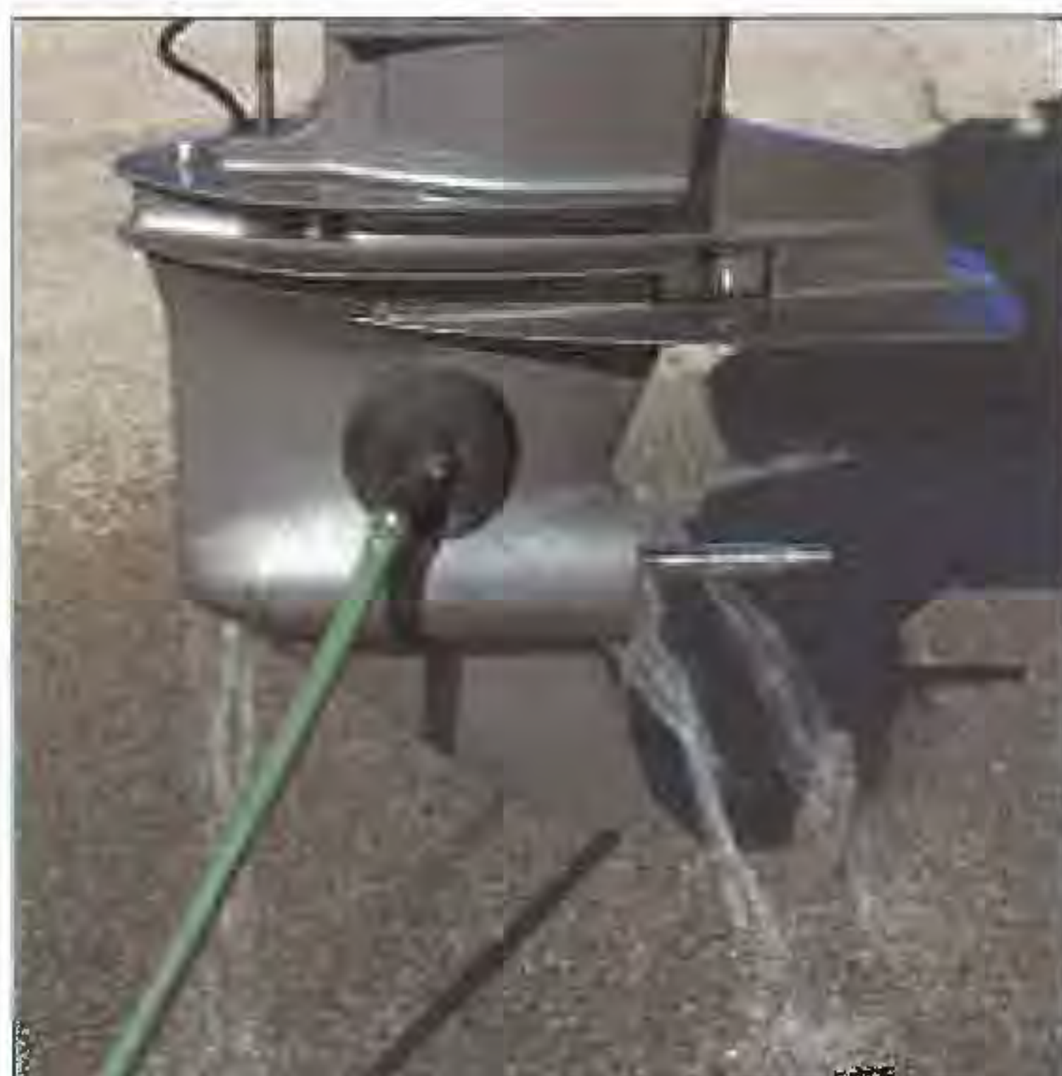
Figure 4-4 Flush motor with fresh water after each salt- water excursion
