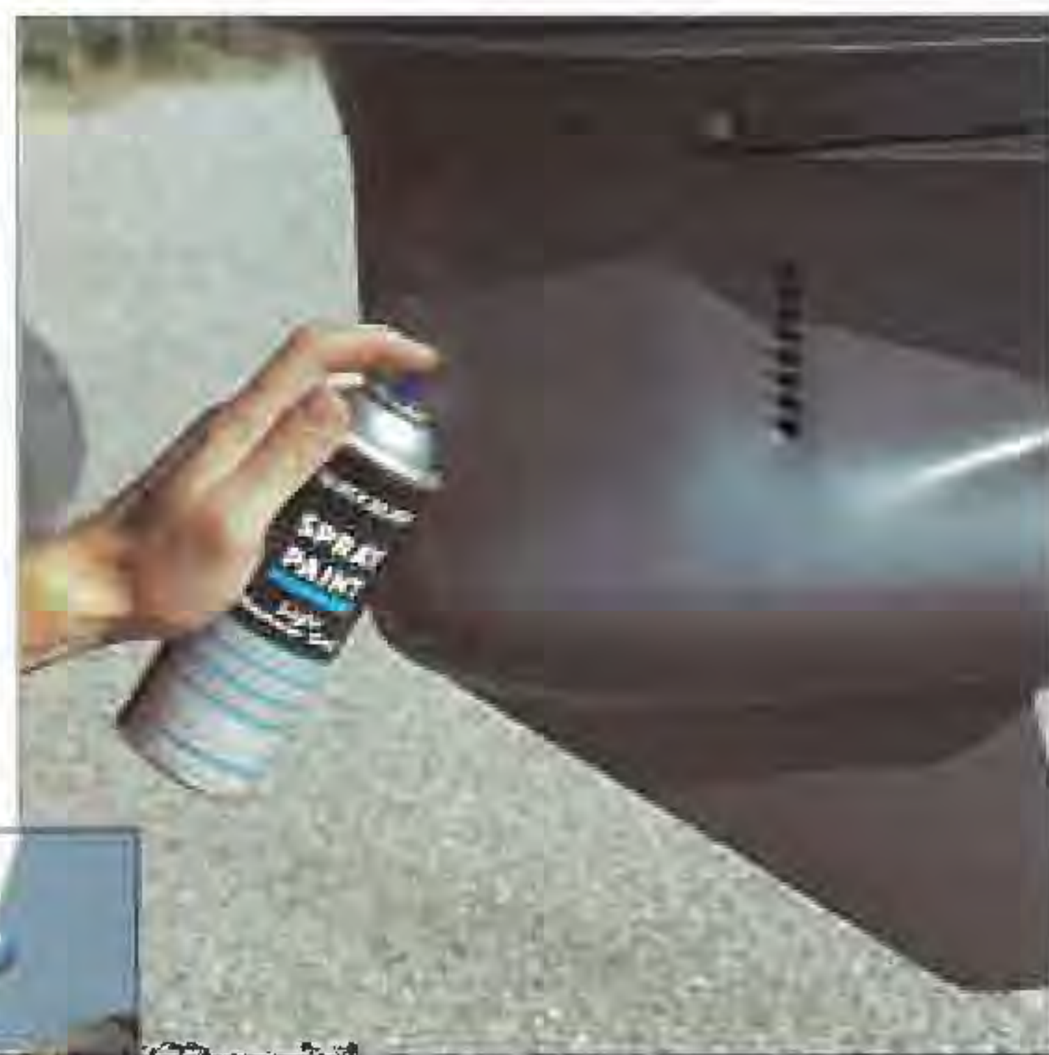
Figure 4-1 Maintain paint coverage on lower unit
