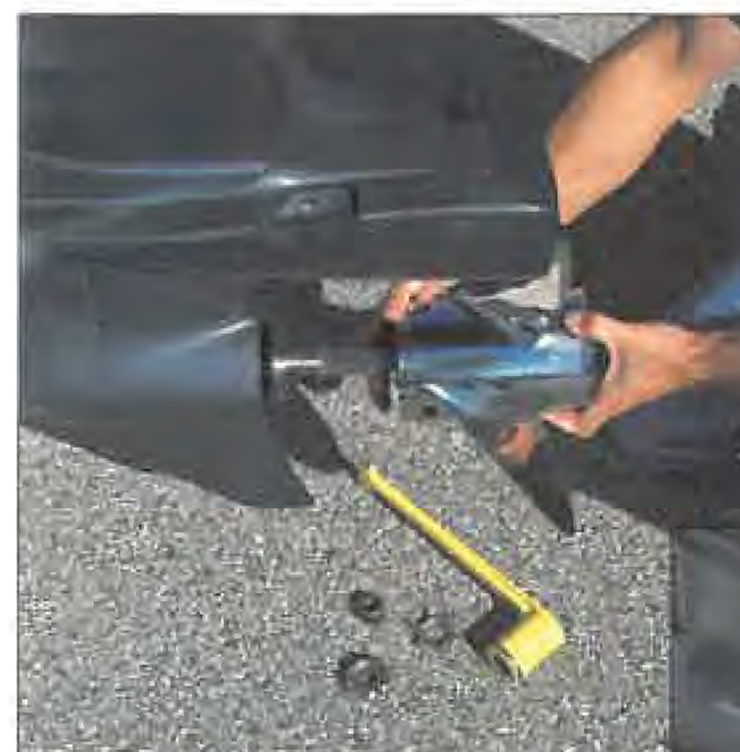
Figure 4-7 Propellers should be removed and propeller shaft lubricated every 60 days
