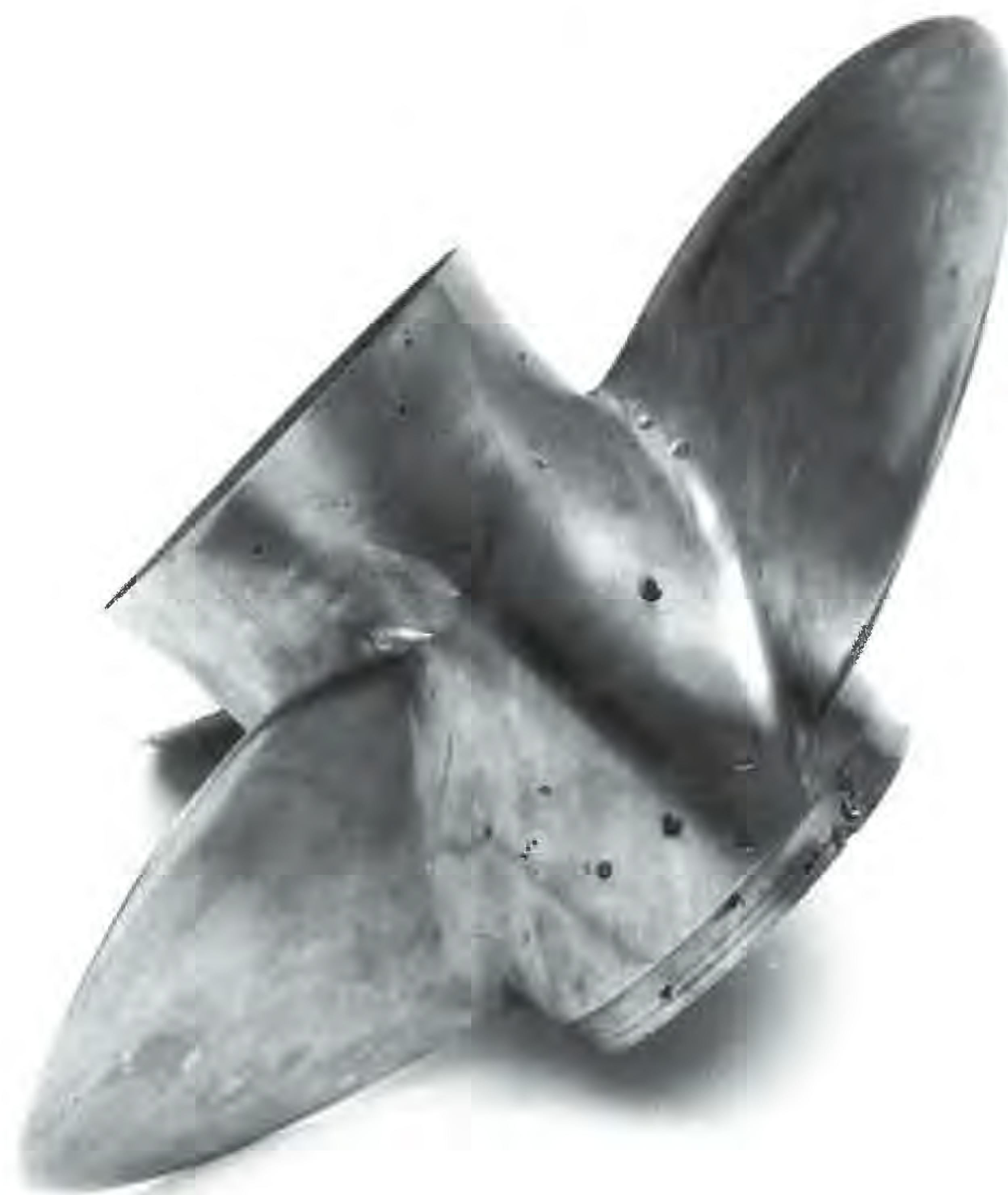
Figure 3-16 Propeller corrosion from loss of continuity
