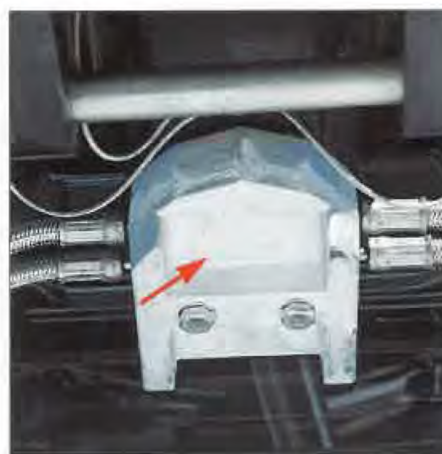
Figure 2-7 Drive-mounted sacrificial anode (MerCruiser anodic block on drive)
