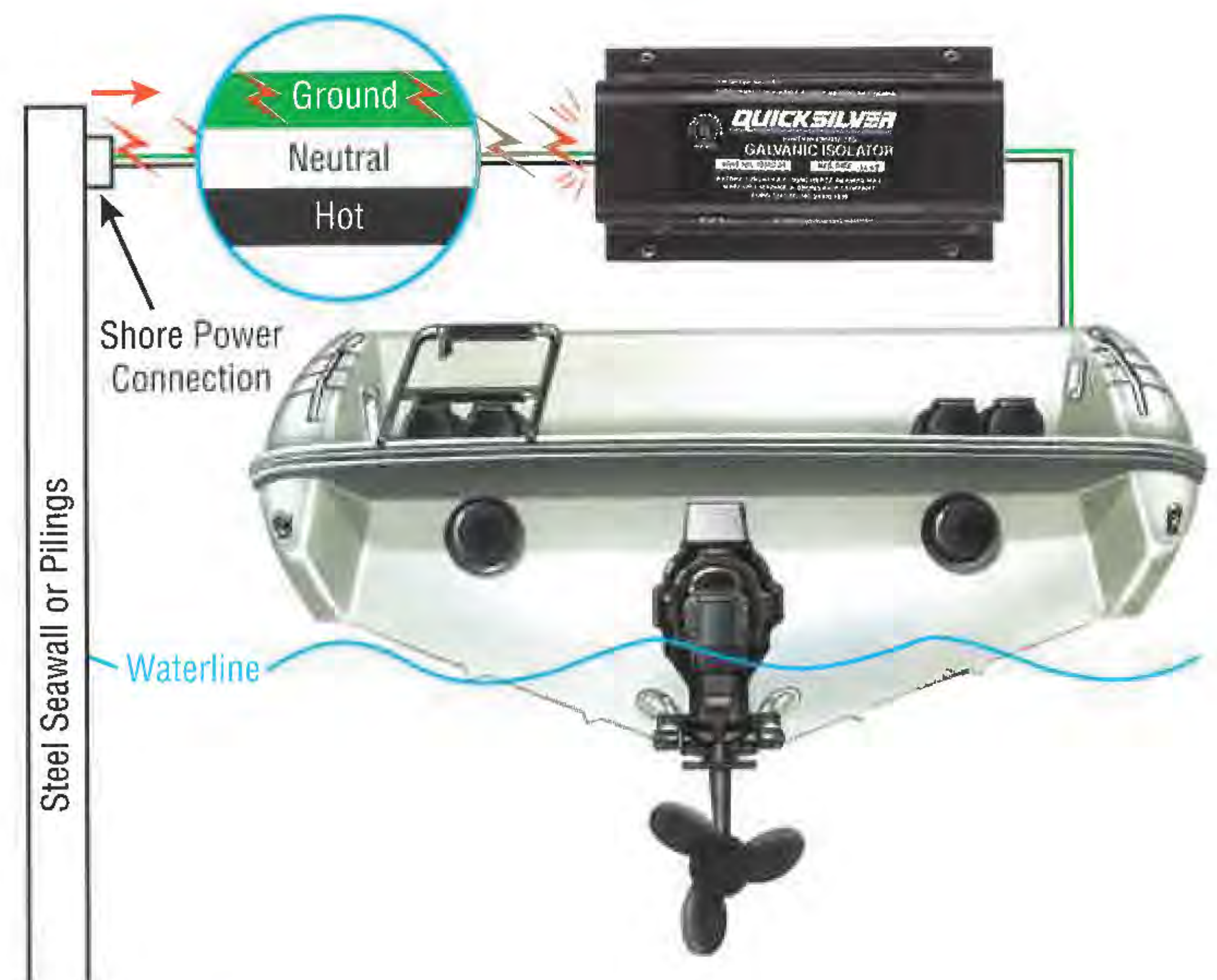
Figure 2-26 Galvanic current flow with isolator
