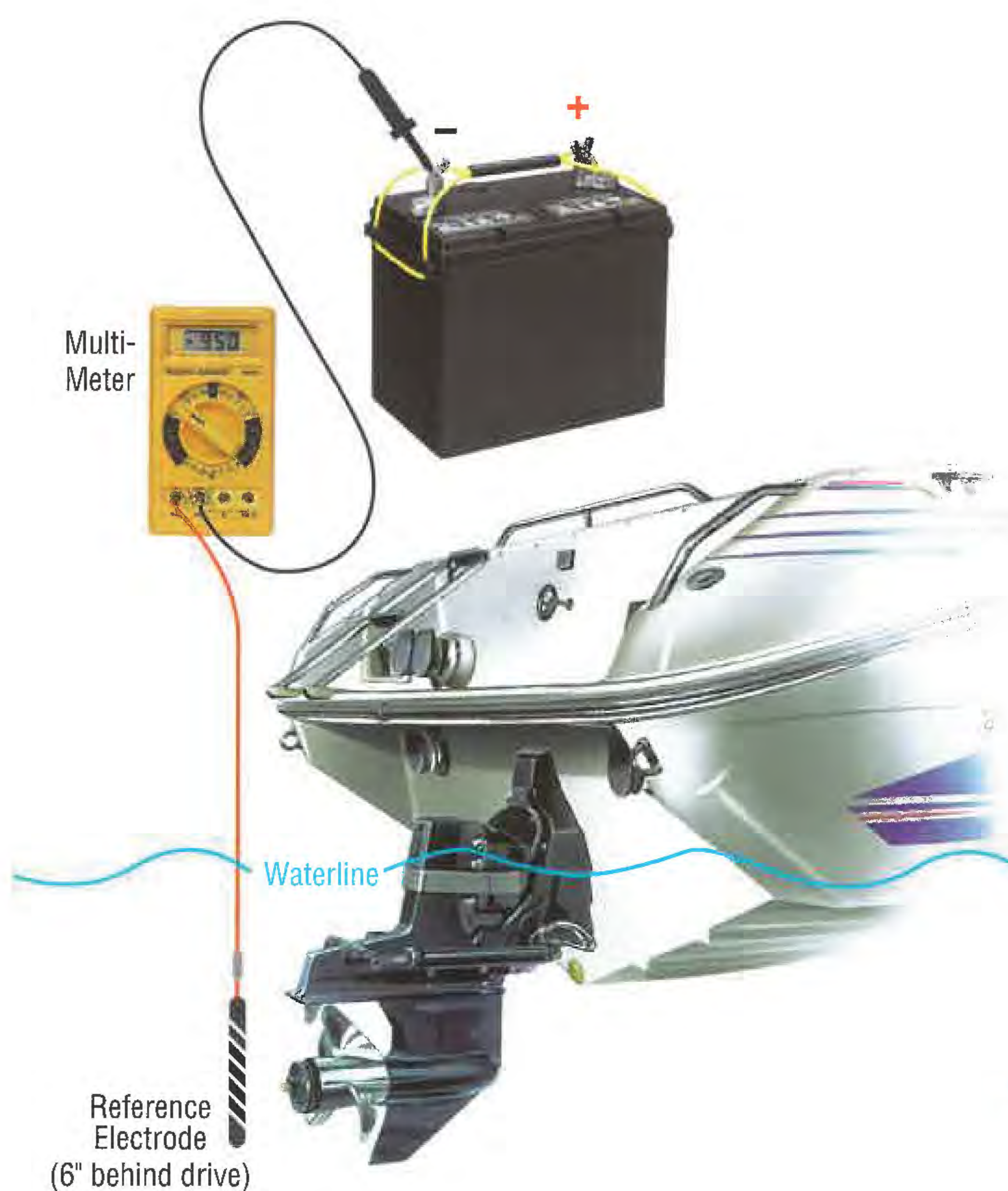
Figure 3-1 Reference electrode tester positioned properly
