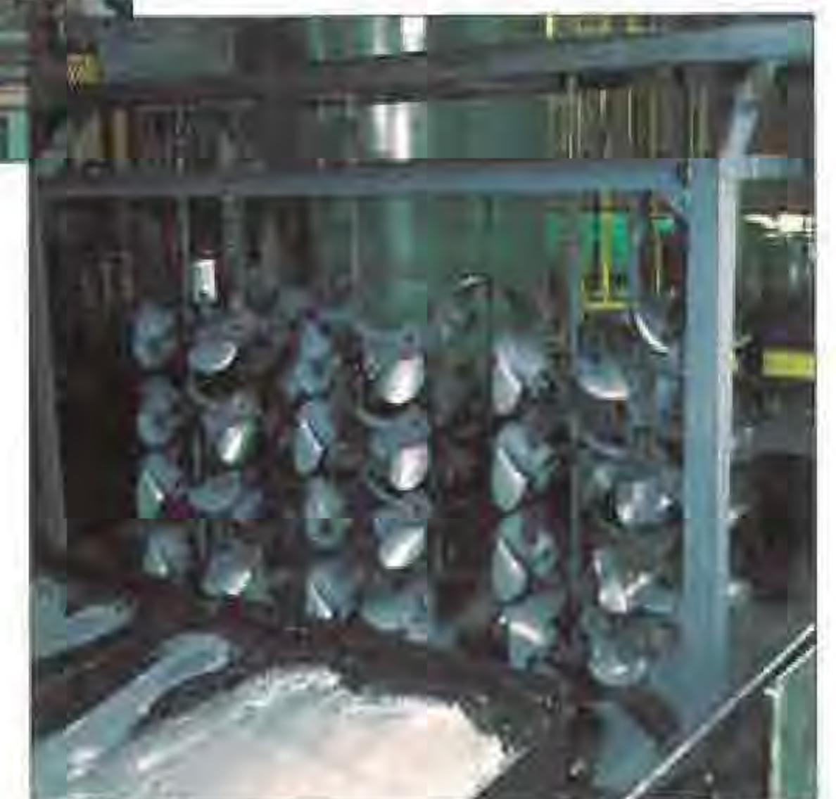
Figure 2-2 Aluminum alloy parts receiving electro-deposited paint (EDP)
