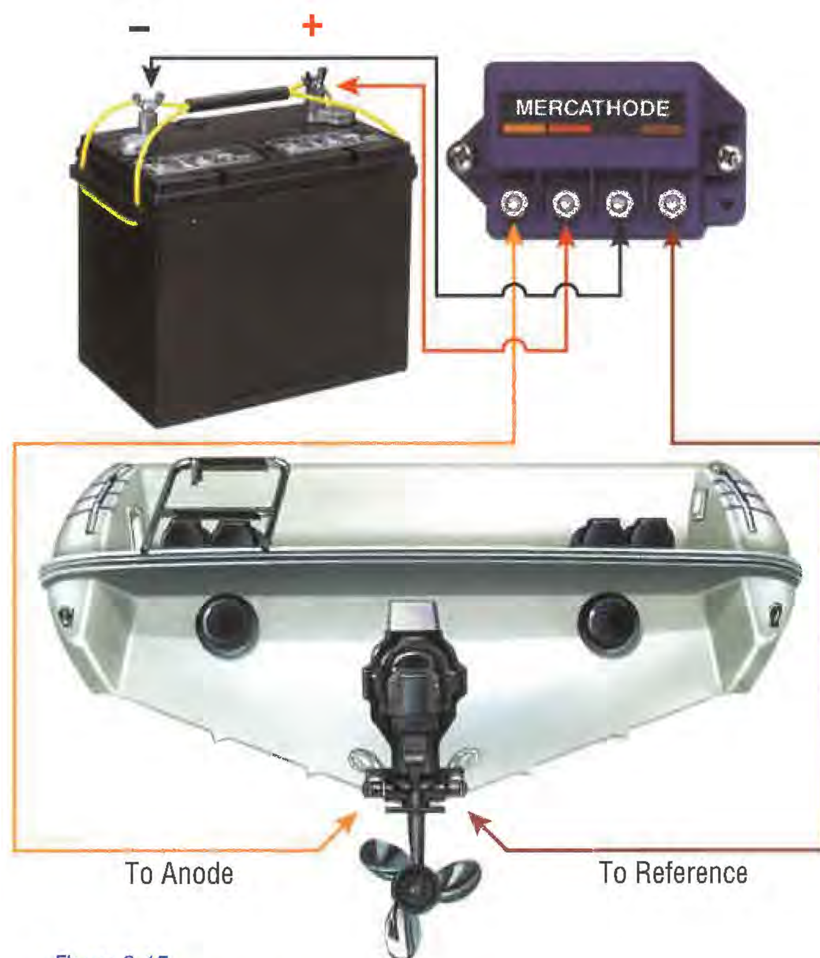
Figure 2-15 Quicksilver MerCathode System installation
