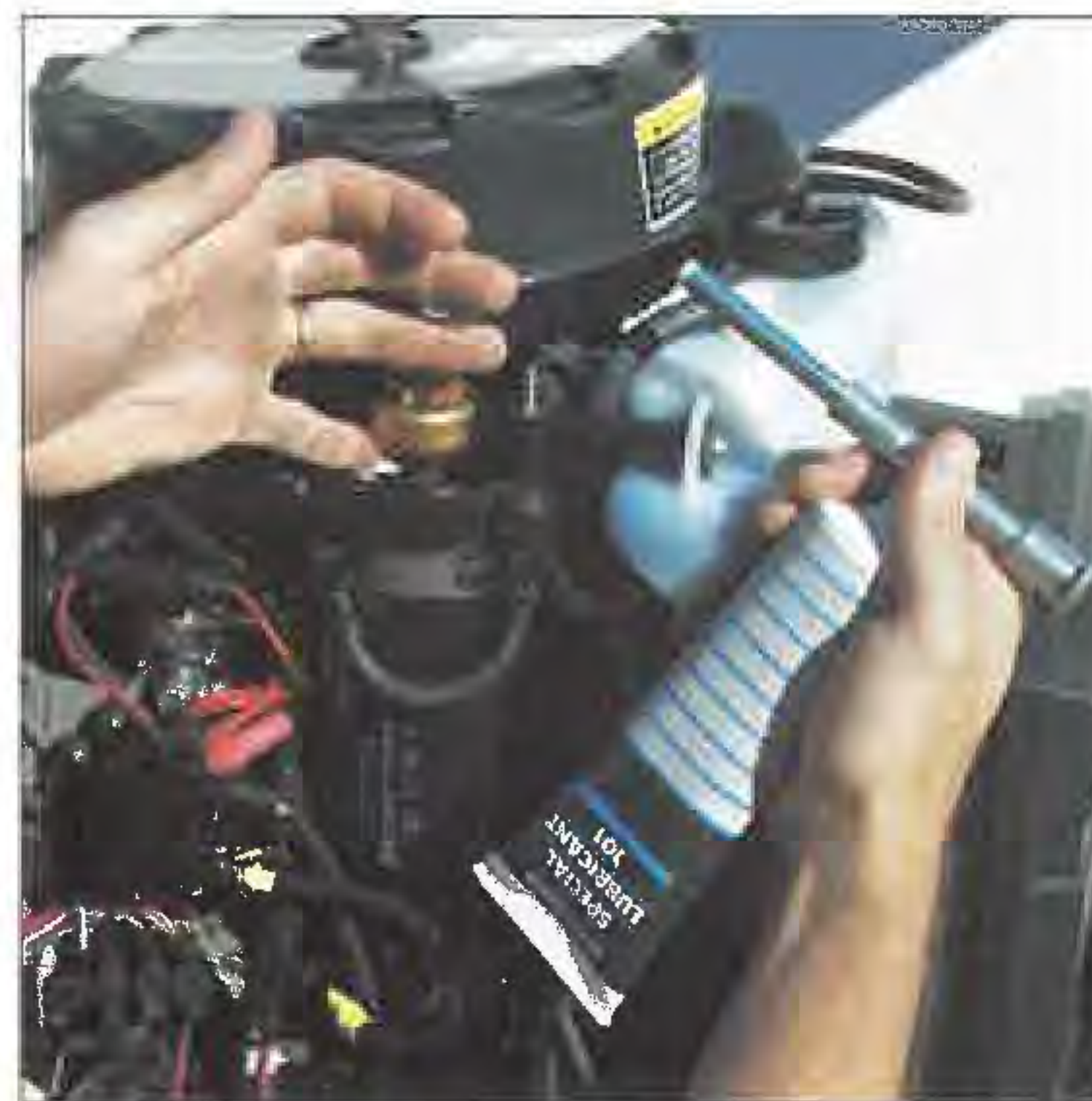
Figure 4-8 Lubricate other points such as starter motor pinion shaft
