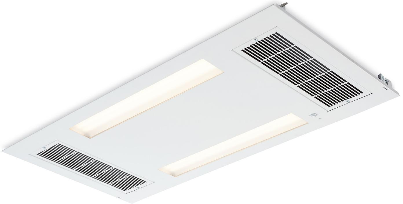
Routine maintenance to key components of the Cleanse Retrofit Troffer will help to sustain peak performance and minimize downtime. For optimal performance, HEPA/Charcoal filter should be inspected monthly and is recommended to be replaced every six months. For UV LED, it is recommended to replace after every 2,000 hours of service as indicated by a solid yellow indicator light on the Troffer.
