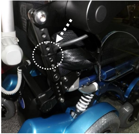
010 Use cable tie to fixed cable
