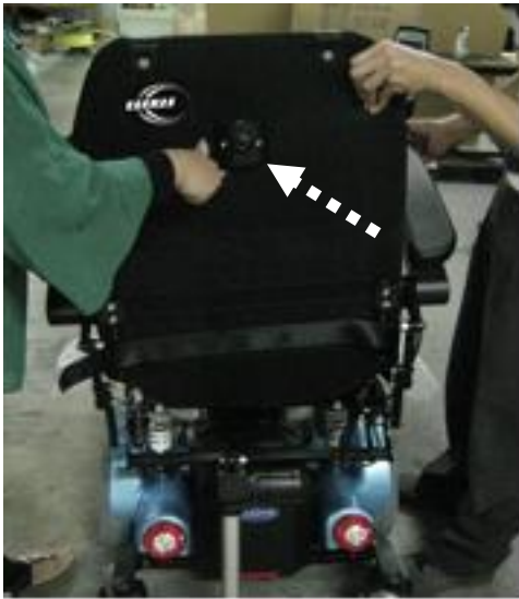
003 After the back cushion to stop positive ,Align the hole and tighten screws ( Not too tighten )
