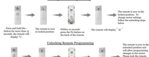
Press and hold the - button for more than 15 seconds, the remote will display "U" The remote is now in the unlocked position
