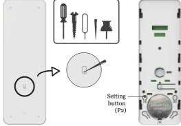
To remove the back cover, use a tool such as a sim card pin, mini screwdriver or paper clip. Press down on the center of the hole on the backside and simultaneously slide the cover in a downward movement.
