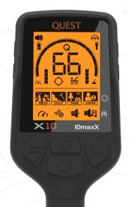
**WORKING METHOD:** 12kHz VLF (Very Low Frequency)
