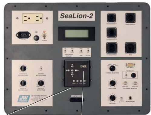
Control Panel layout with built-in DVR
