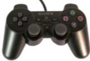
A PS2 Controller's joystick and buttons control the ROV
