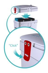
Place the compression handle back on the lid by stretching it over the attachment points on each side of the AirBuddy.
