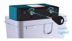
Always care about the battery terminals and lugs. Prevent any contact with water (leading to oxidation), mechanical damage (e.g. scratches) or dirt (e.g. grease residues) that could impede the electrical conductivity of the connection.
