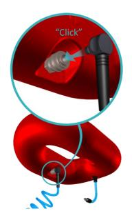
Always make sure that the diver's hose is properly connected to the air reservoir. You must hear a "click" sound and you can't pull the hose back.
