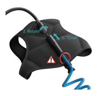
Always check that the diver's hose is properly connected to the air coupler on the harness and you can't pull it back. Always rotate the sleeve of the coupler to lock the diver's hose. Visually check the coupler to make sure that the notch (on the coupler sleeve) is on the opposite side than the pin (on the body of the coupler).
