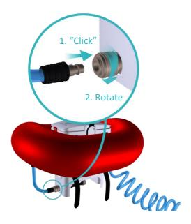
Push the plug into the air coupler until you hear an audible "click" sound and you can't pull it back. This coupler is fitted with a lock to prevent an accidental release of the hose. Rotate the sleeve of the coupler to misalign the pin with the notch.
