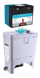
Unscrew the two stainless steel button-head screws from the battery and connect the battery wires. Place the lugs over the battery main terminals and fasten the screws with a 4mm hex
