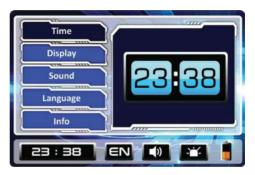
press the right key, and use the up and down keys to adjust the minutes.
