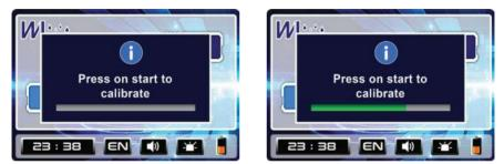
**Note:** In order to reset the calibration, press the start button on the handle and wait 5 seconds for the reset process to complete. Always try to keep the device horizontal.
