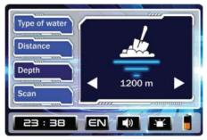
Use the left/right keys on the keyboard to change the desired depth. We also always recommend choosing the appropriate distance for the area in which we are searching, meaning it is not necessary to always choose the largest distance value available in the device.
