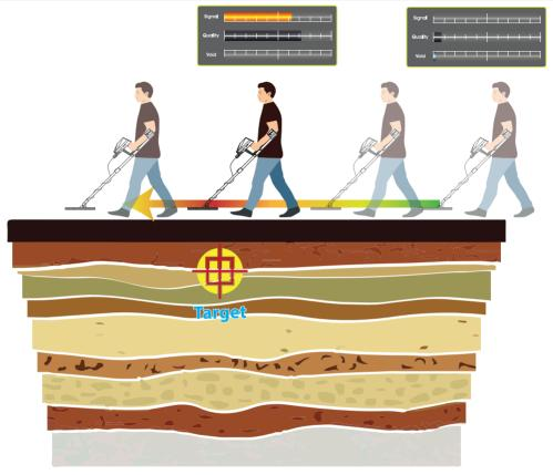
While moving over the scan area track the changes on the display in the Signal, Quality and Void levels and reading intensity to enclose targets.
