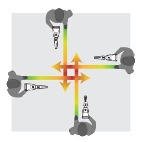
Once the target point is enclosed and located, mark it and proceed to the Depth measuring process next.
