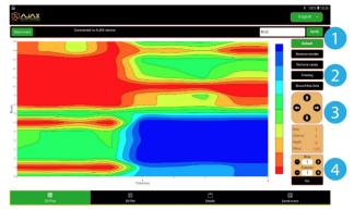
The 3D plot shows a three-dimensional surface representing the scan data values.
