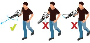
Face the targeted search area and wait for the device to receive a signal indicated by the antennas moving towards targets directions.
