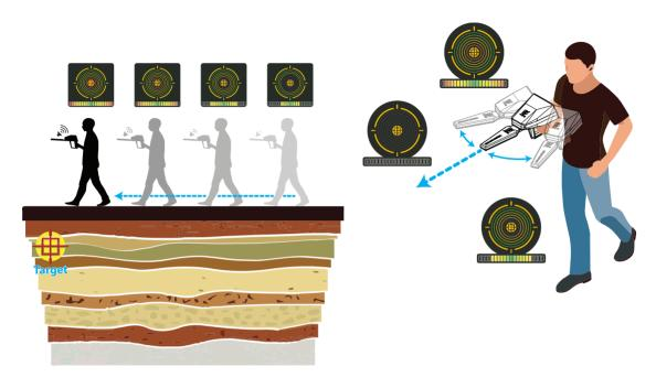
Hold the device horizontally and move it right and left until a signal indicating a probable target is received.
