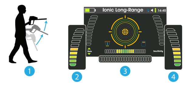
The device should be balanced with the ground value before proceeding into the search.
